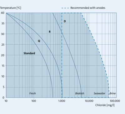
pump configuration. Contact Grundfos for an evaluation of your conditions, and for anode options.
