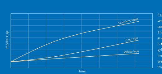
Cast iron has very good wear rate, even when compared to white iron. The unique groove in the suction cover of the open S-**tube**<sup>®</sup> minimises the grinding effect on the impeller caused by material wedged between the impeller and suction cover.
