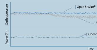
The following comparison shows Open S-tube® and suction cover in action during an accelerated clogging test. The Open S-**tube®** is being compared to an alternative "self-cleaning" open impeller. Self-cleaning hydraulics typically accumulate fibers until they are released, resulting in a continual part blockage which negatively affects its performance.
