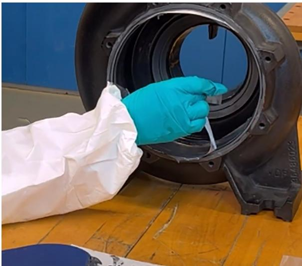
13. Immediately remove masking tape and shape edges while coating is still malleable.
