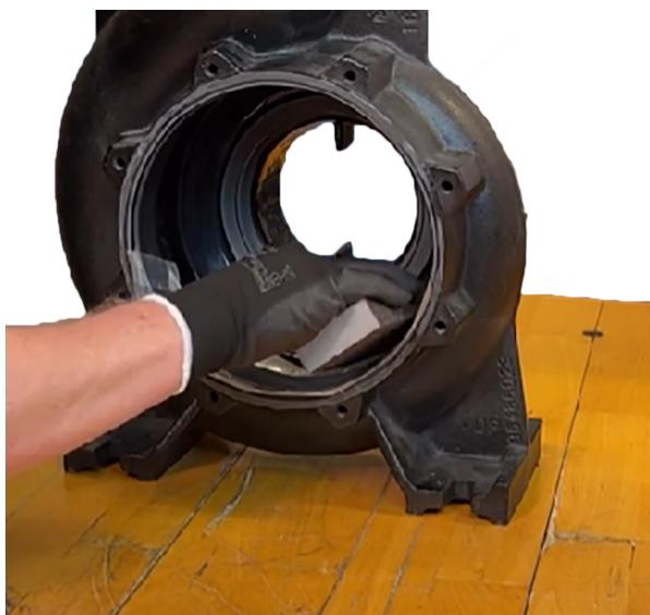
3. Remove the first round of masking tape. Now, all particles from the grinding can be removed.
