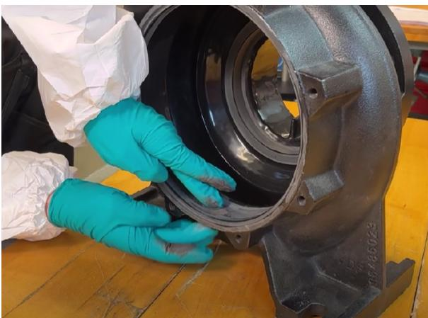
8. Apply the repairing coating to external surfaces and cover a larger area than the damaged area, to ensure proper adhesion and strength.
