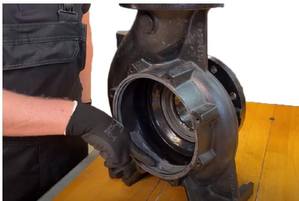
1. Make sure that the rusted and damaged areas are removed by grinding/machining.
