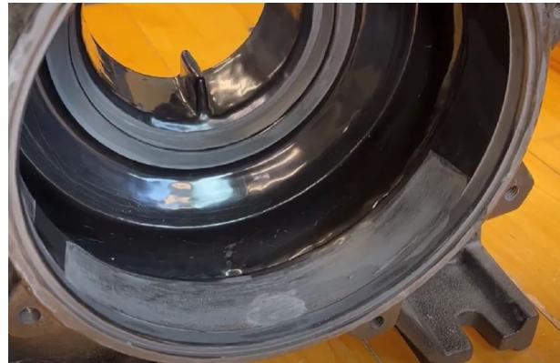
5. Degrease and remove residues from the grinding.
