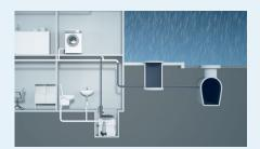
**Lifting station (inside buildings)** Installed in a tank solution in basements and other building spaces below sewer level.
