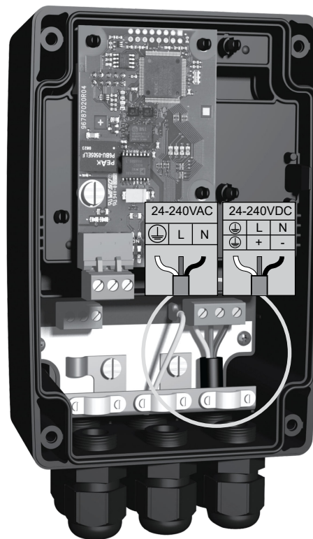
Electrical connections, CIU 903
