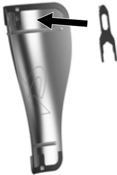
Fig. 3 Fitting adjusting fork D on the backside of coupling guard (7)
