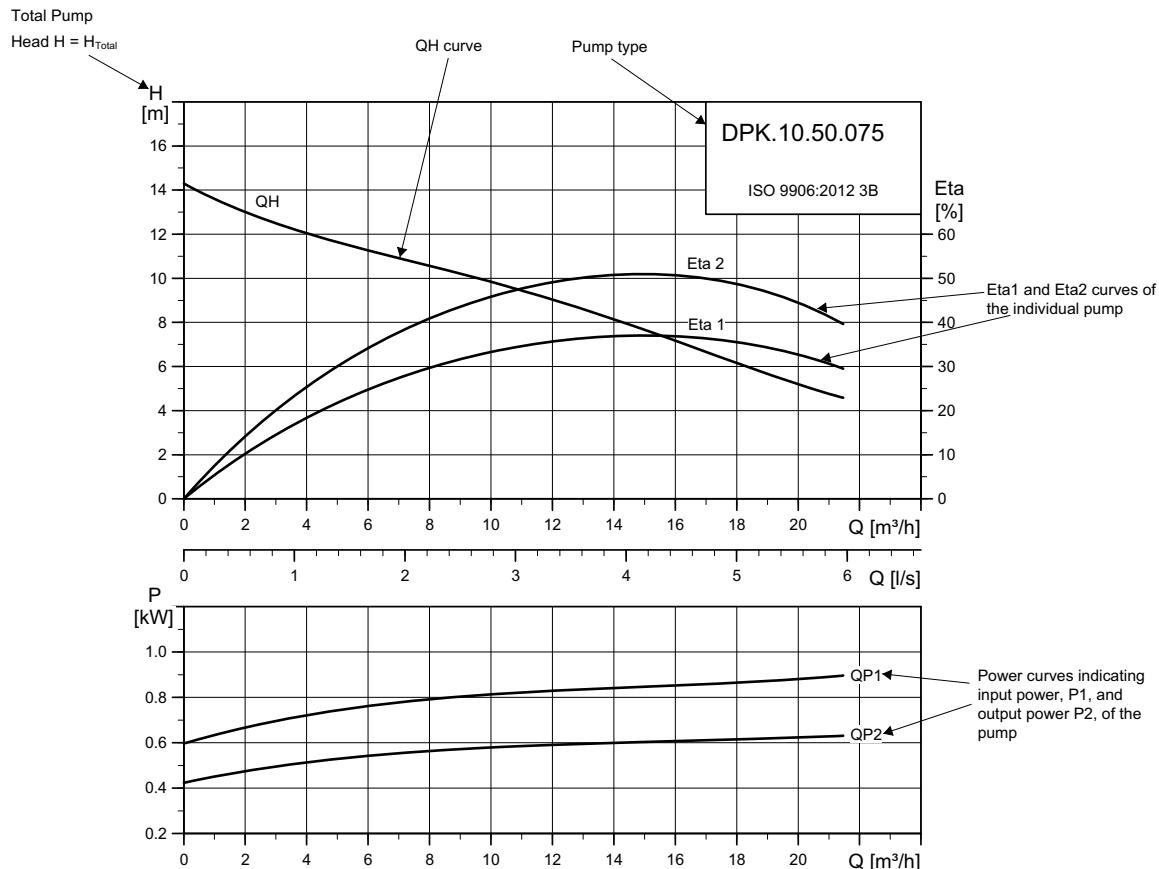
**Note:** The pumps are tested according to ISO 9906:2012 grade 3B tolerance. Testing equipment and measuring instruments are designed and calibrated according to this standard. The pumps are approved according to tolerances for entire curves, specified in grade 3B.
