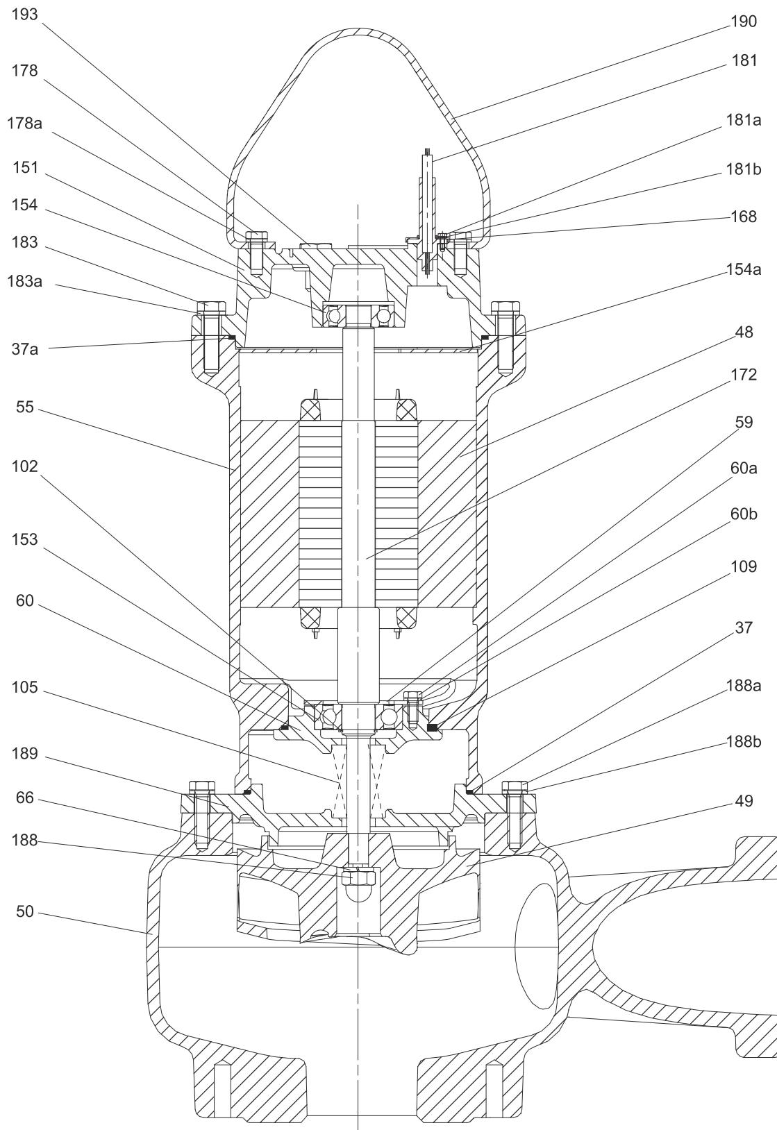
**Fig. 20** Sectional drawing DPK.V.65.80.15.2 and DPK.V.65.80.22.2
