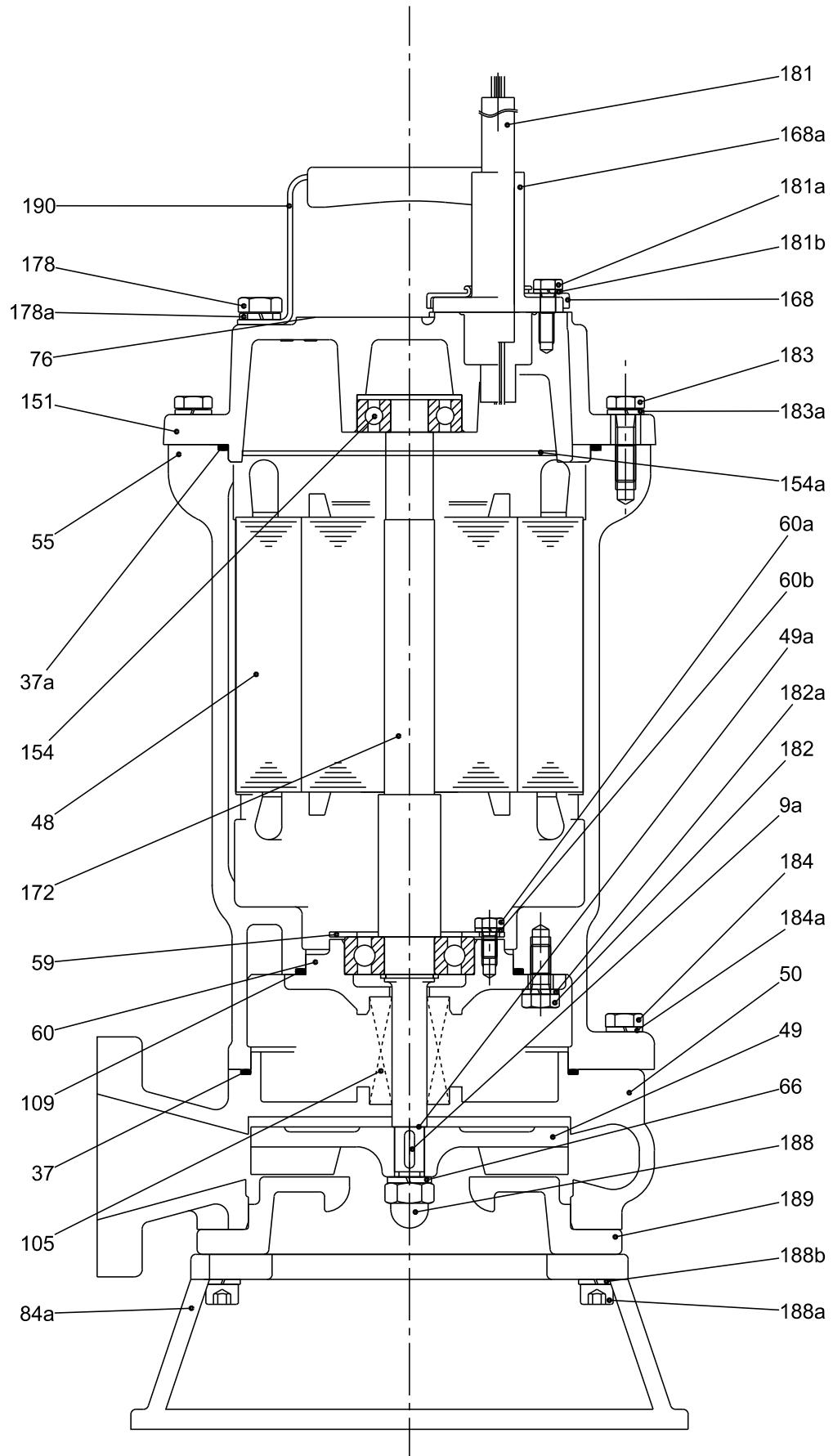
**Fig. 9** Sectional drawing DPK.10.50.075 and DPK.10.50.15
