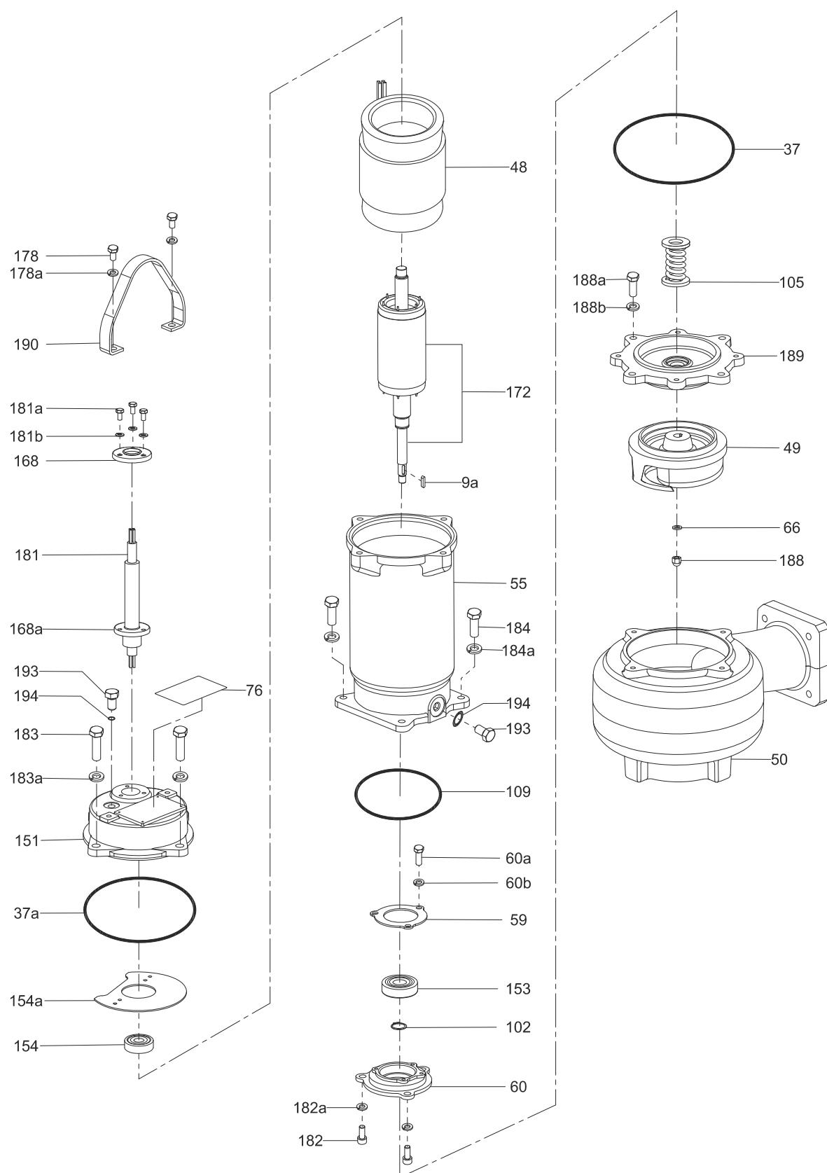
Fig. 19 Sectional view DPK.V.65.80.15.2 and DPK.V.65.80.22.2
