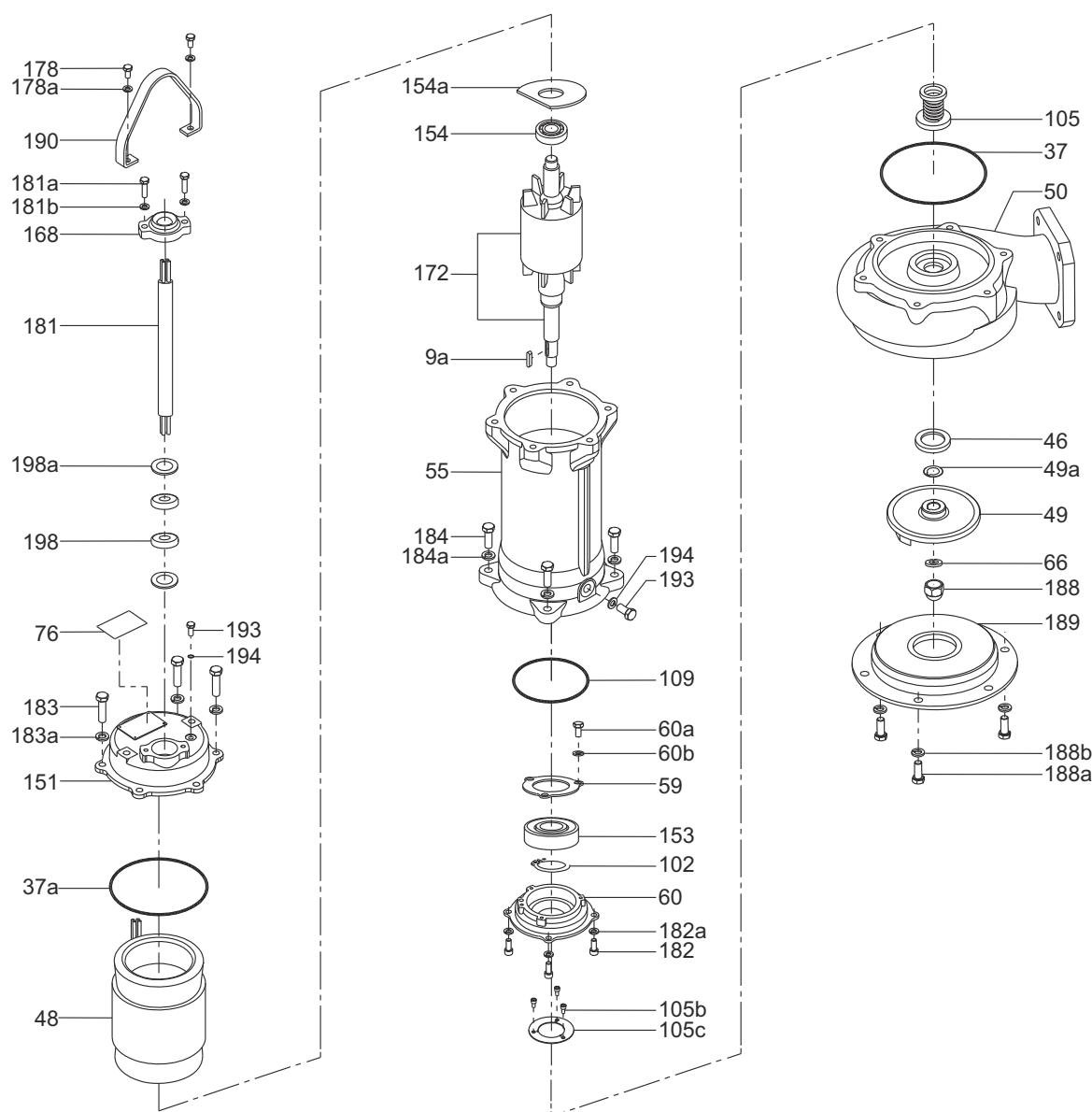
**Fig. 13** Exploded view DPK.15.80.37, DPK.15.100.55, DPK.15.100.75, DPK.20.100.110 and DPK.20.100.150
