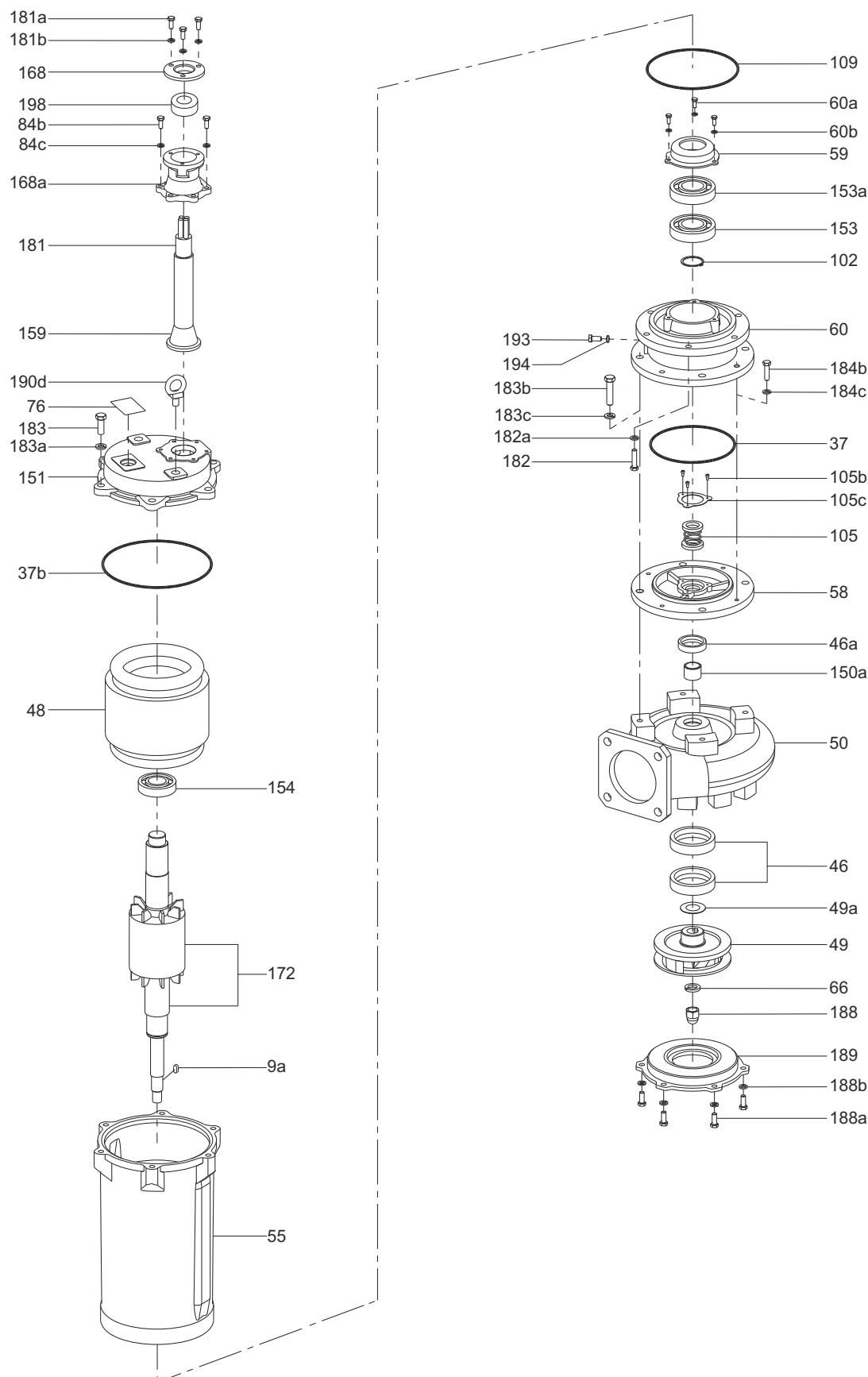
Fig. 17 Exploded view DPK.20.150.190 and DPK.20.150.220
