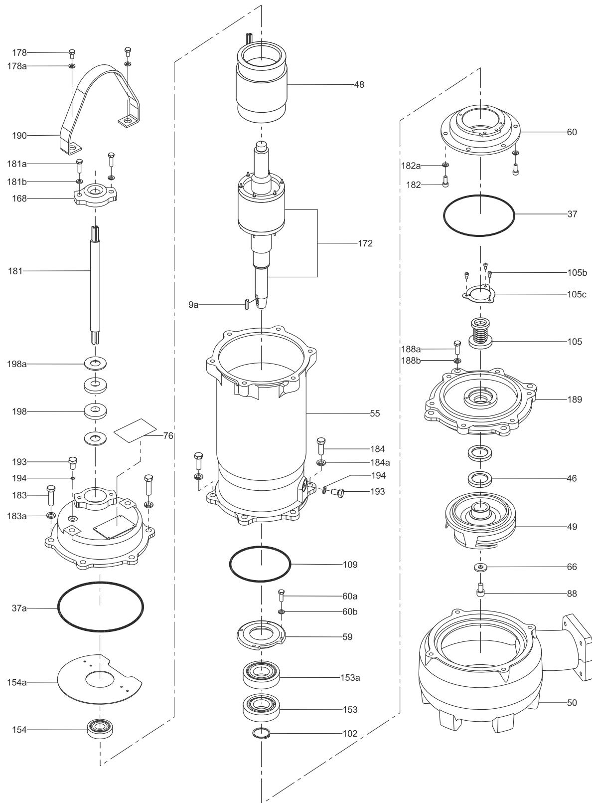
**Fig. 23** Exploded view DPK.V.80.80.55.2 and DPK.V.80.80.75.2
