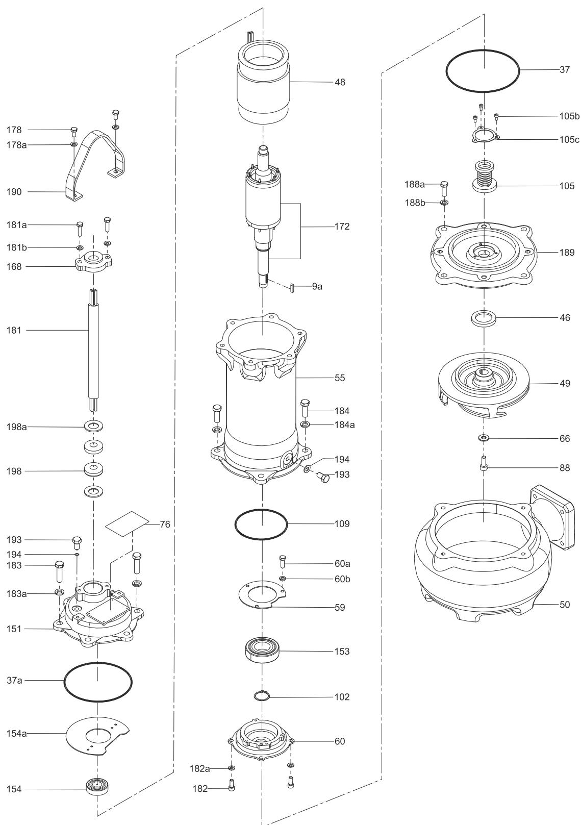
Fig. 25 Exploded view DPK.V.65.80.15.4 and DPK.V.65.80.22.4
