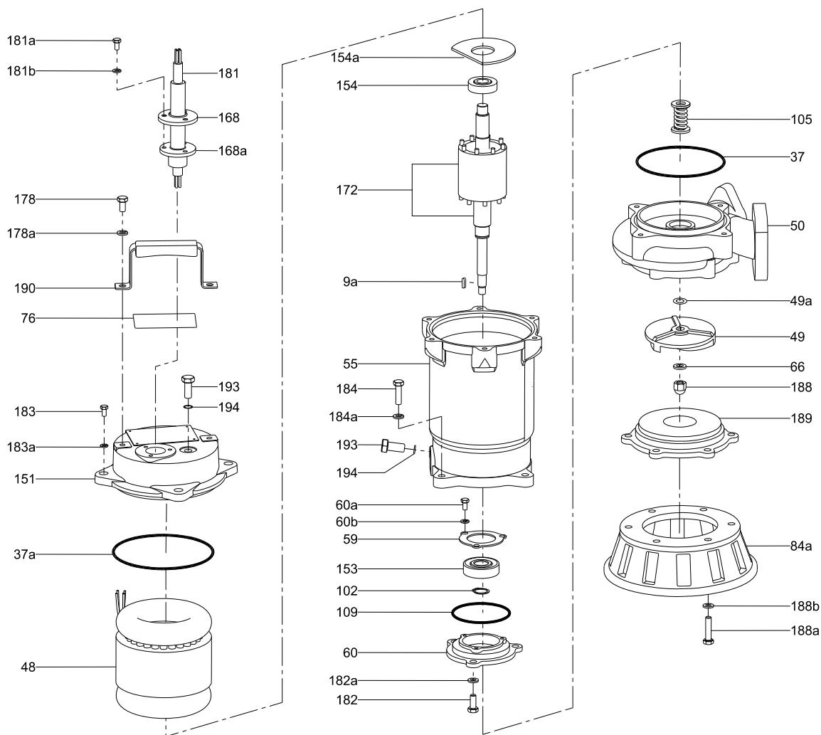
**Fig. 8** Exploded view DPK.10.50.075, DPK.10.50.15 and DPK.10.80.22
