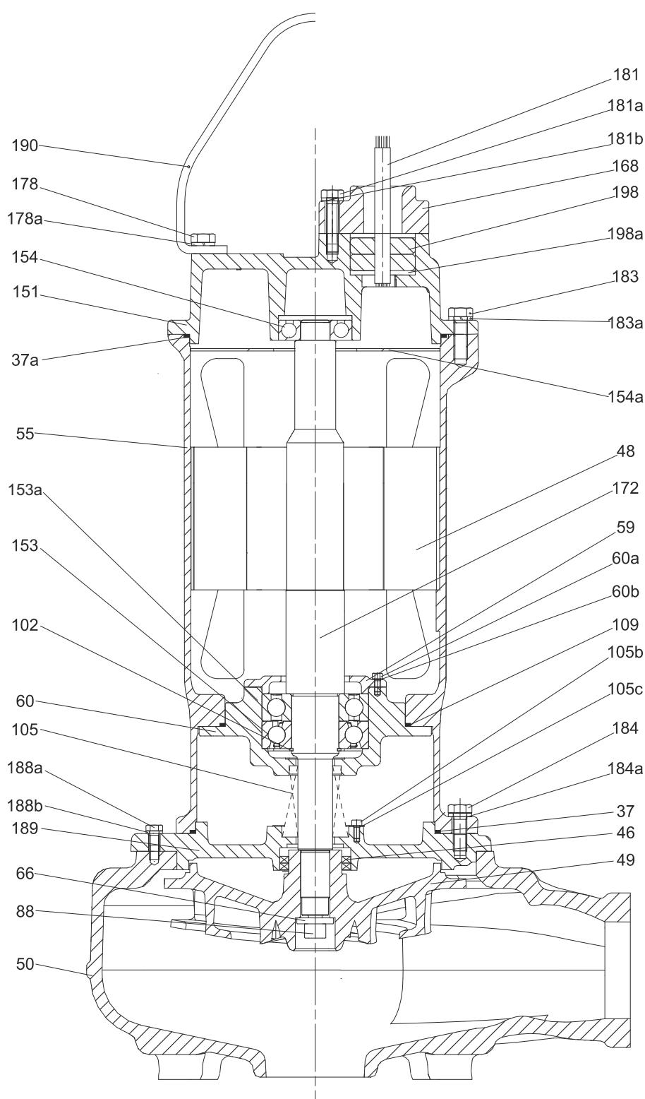
**Fig. 28** Sectional drawing DPK.V.80.80.37.4, DPK.V.80.80.55.4 and DPK.V.80.80.75.4
