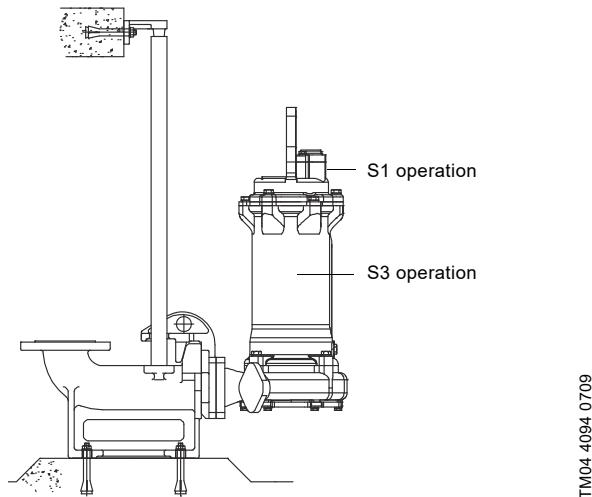
**Fig. 29** Liquid level for DPK pumps in S1 or S3 operation
