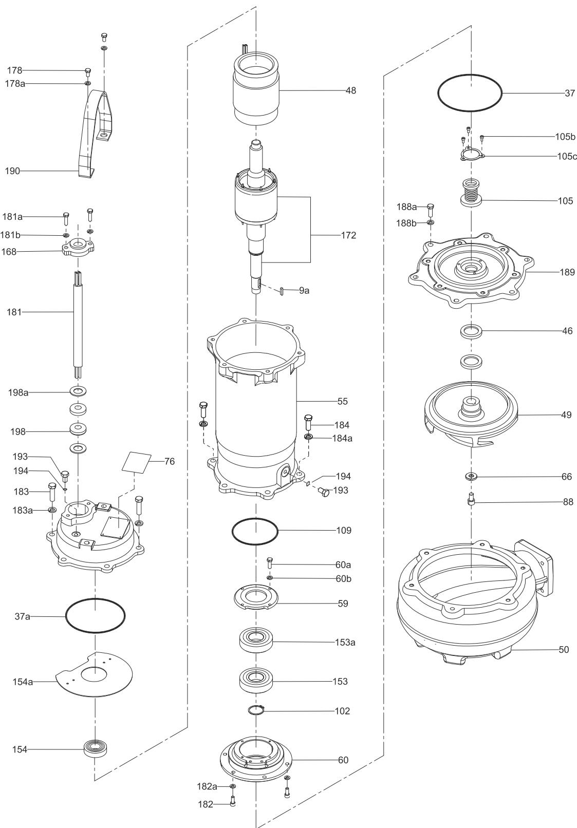
**Fig. 27** Exploded view DPK.V.80.80.37.4, DPK.V.80.80.55.4 and DPK.V.80.80.75.4
