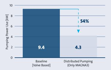
Replacing the balance and control valves with distributed pumps reduced the total pump energy consumption for the chilled water loop by 54%.
