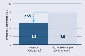
The design Delta T is 7 °C. Before the distributed pumping concept, its Delta T was 5.3 °C, which increased to 7.8 °C after introducing the concept.
