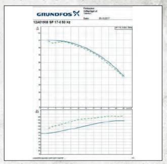
**Conclusion:** The curve shows that to maintain a flow of 17m³, power consumption has increased by 1 kW. With a pumping requirement of 9 hours per day, that equates to **3,285 kWh over a year,** or a **16 % increase** in energy use.
