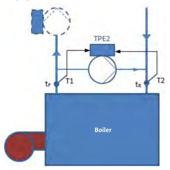
Temperature sensors/transmitters 0-150  $^{\circ}$ C / 4-20 mA are installed in the supply and return pipes respectively. The , return temperature sensor is placed at the bottom of the boiler.
