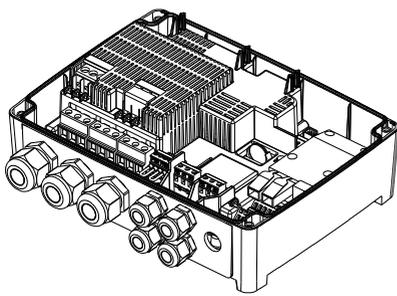
**!** Do not tighten the cable glands too much since this may damage the rubber seals.
