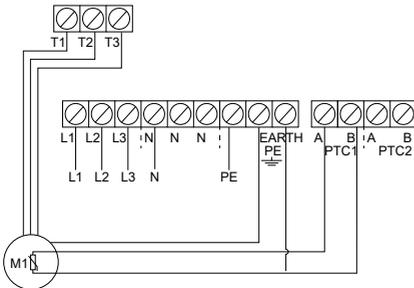
*Three-phase connections for one pump*
