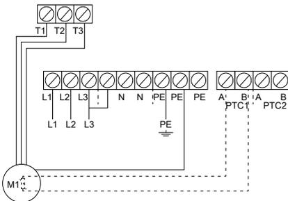
*Three-phase connections for one pump without neutral, for Norway only*
