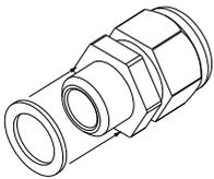
2. Mount the cable glands on the control unit.
