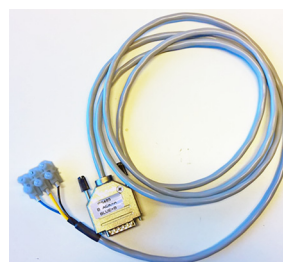
Fig. 8 RS485 cable with screw terminal connector from PC Tool Link package
