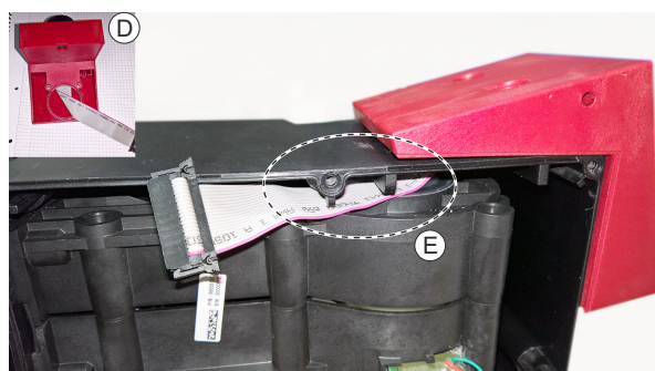
Fig. 6 Control cube cable placement
