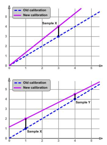
A linear calibration changes the offset and the slope (see figure on the right).
