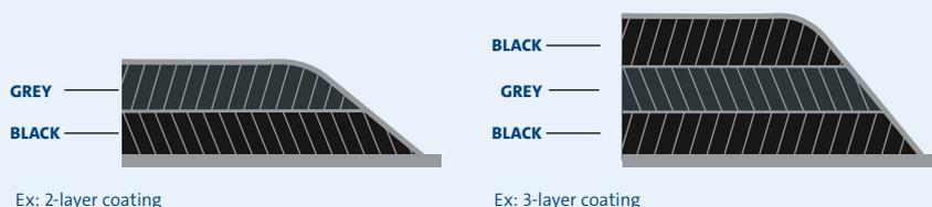
As layers are always applied in different colors (each layer having the same physical properties) it is easy to spot if there are areas in the pump that are exposed to wear or has been damaged. If the top coat is partially worn or damaged, it is time to consider when to make your next move. . If the wear is severe and metal is exposed to corrosion, consider a complete recoat of the pump.
