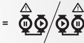
One pump is operating continuously. The backup pump is operated at intervals to prevent seizing up. If the duty pump stops due to a fault, the backup pump will start automatically.
