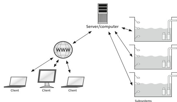
Figure 62 Illustration of the principle in web-hosted SCADA
