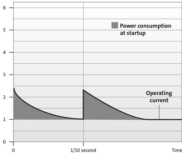
Figure 34 Current flow by autotransformer starting
