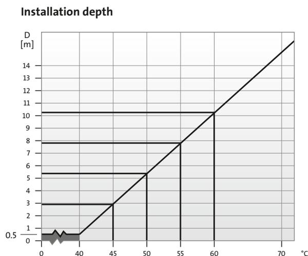
Figure 58 Required water temperature/installation depth of MS 4000 and MS 6000
