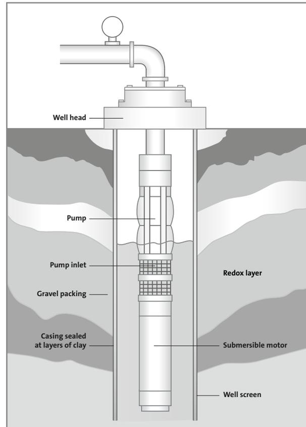
Figure 1 Groundwater well with submersible pump
