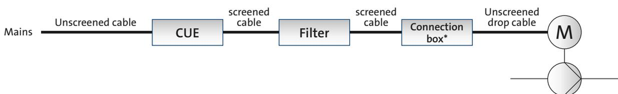
\* Both ends of the screened cable from the filter to the connection box must be connected to earth
