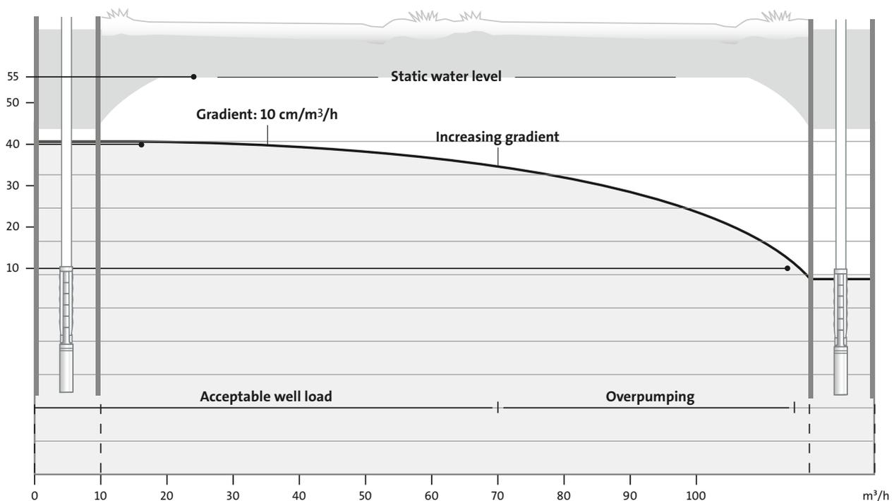
Figure 7 Dynamic water-level variations by test pumping
