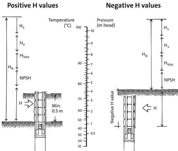
Figure 16 Installation depth
