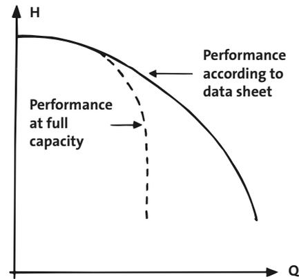
Figure 17 Performance reduction at cavitation
