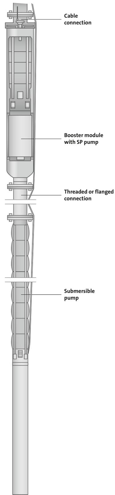
Figure 60 Series coupled submersible pump
