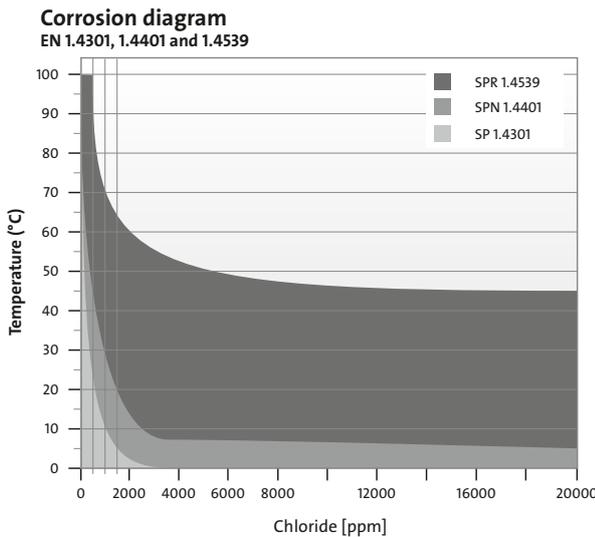
Figure 22 Corrosion diagram
