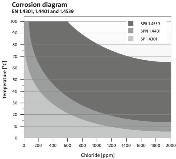
Figure 21 Corrosion diagram
