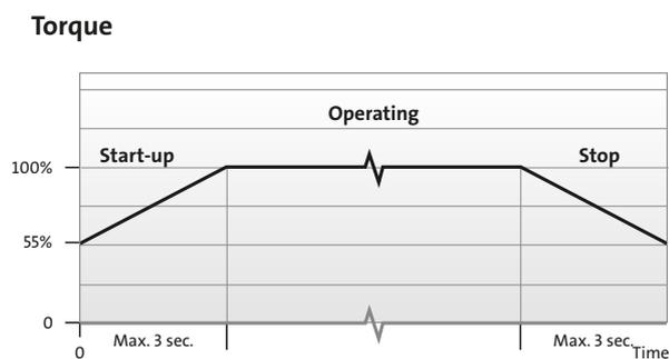
Figure 37 Recommended start-up and stop time, max. 3 sec.
