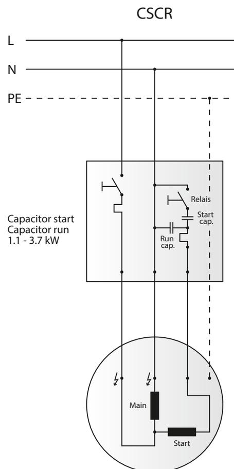
Figure 28 Schematic diagram of a CSCR motor
