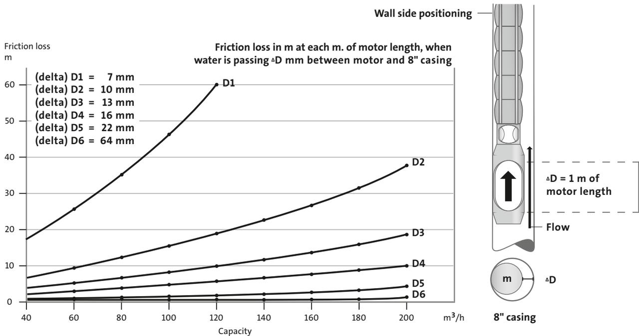
Figure 53 Friction loss, 8"
