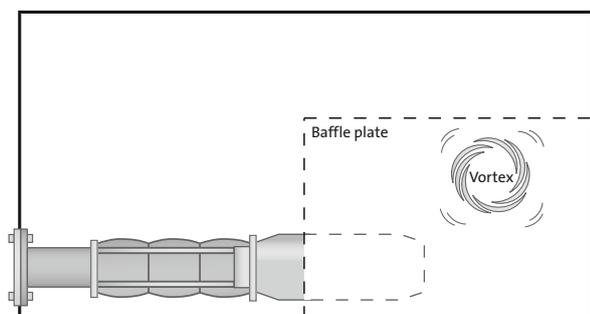
Figure 12 Vortex baffle plate on horizontally-installed pump (seen from above)
