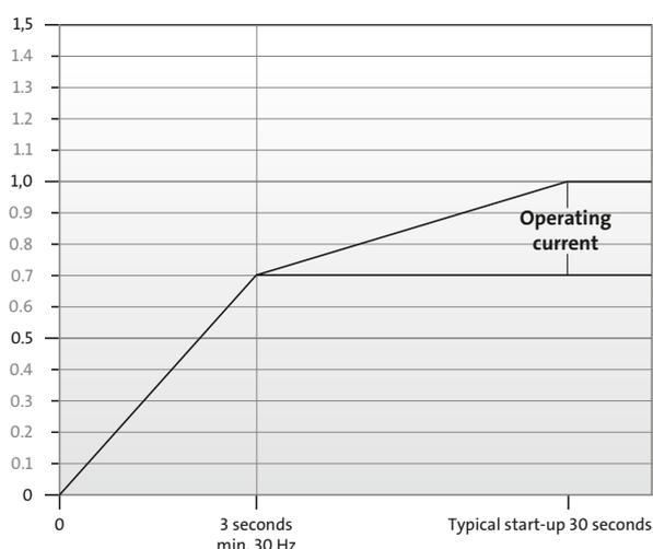
Figure 40 Current flow by frequency converter starting
