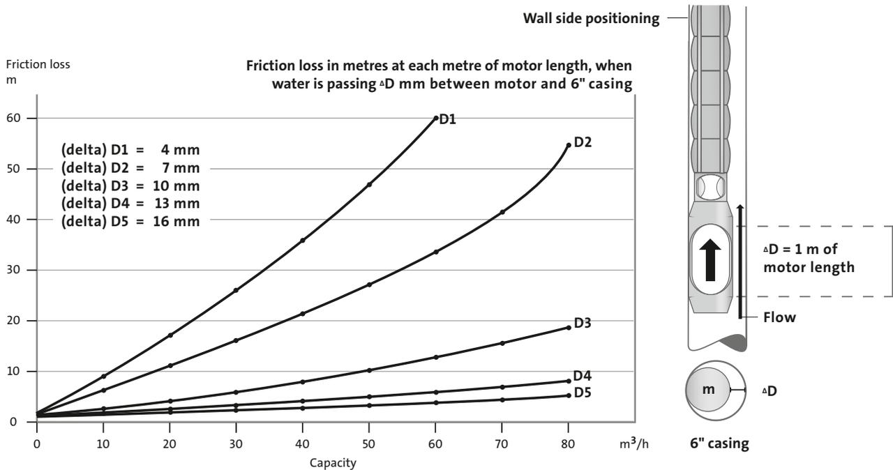
Figure 52 Friction loss, 6"
