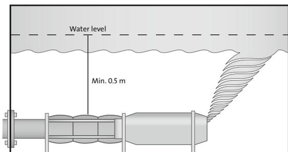
Figure 11 Flow sleeve on horizontally installed pump
