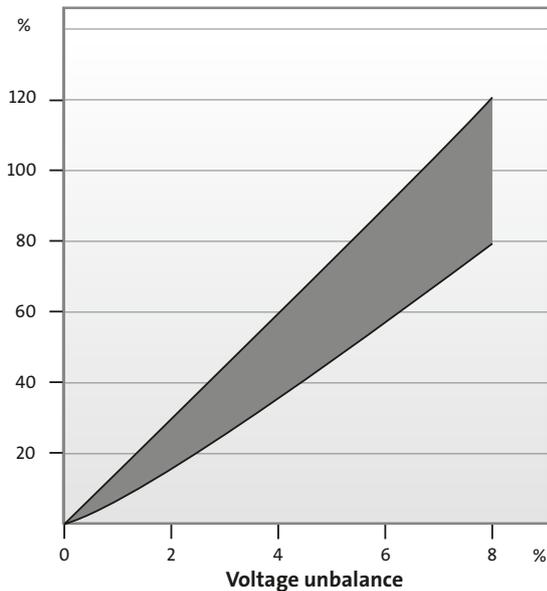
Figure 49 Relationship between voltage unbalance and temperature
