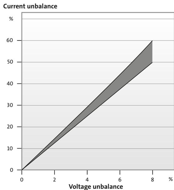
Figure 48 Relationship between voltage and current unbalance
