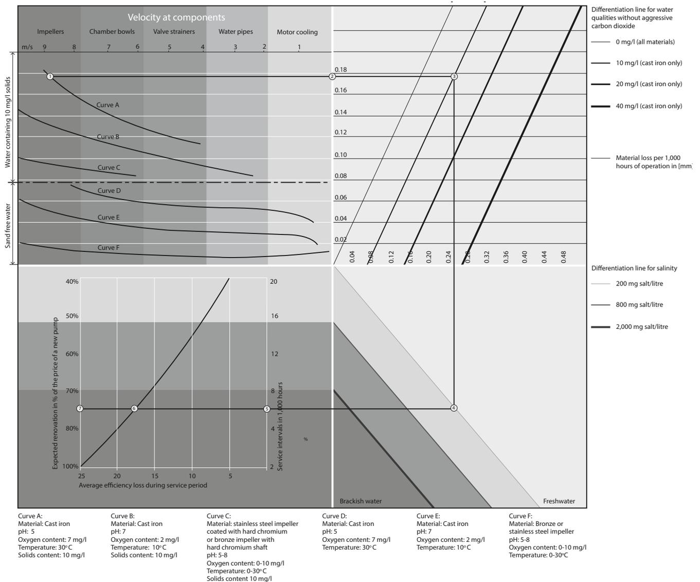
Figure 9 Recommended service intervals for submersible pumps
