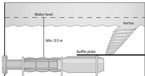
Figure 13 Vortex baffle plate on horizontally installed pump (cross-section)
