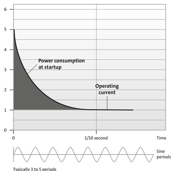
Figure 30 Current flow by DOL starting
