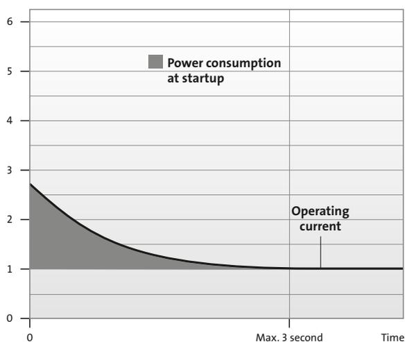
Figure 38 Current flow by soft starting
