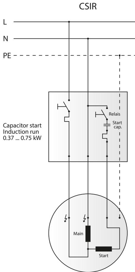
Figure 27 Schematic diagram of a CSIR motor
