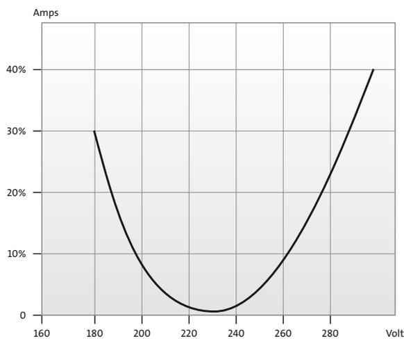
Figure 46 Current variation as a function of over- and undervoltage on a 230 V motor.
