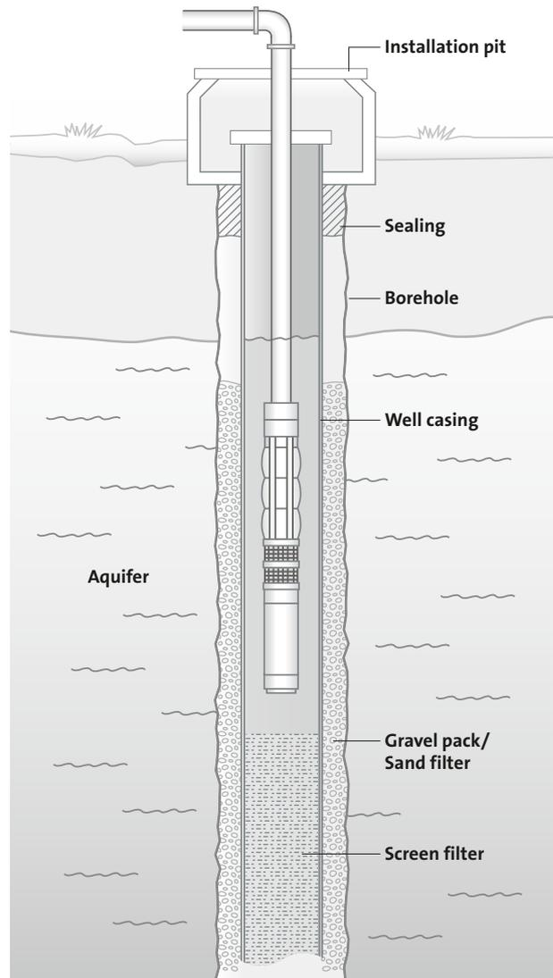
Figure 50 Typical groundwater well components
