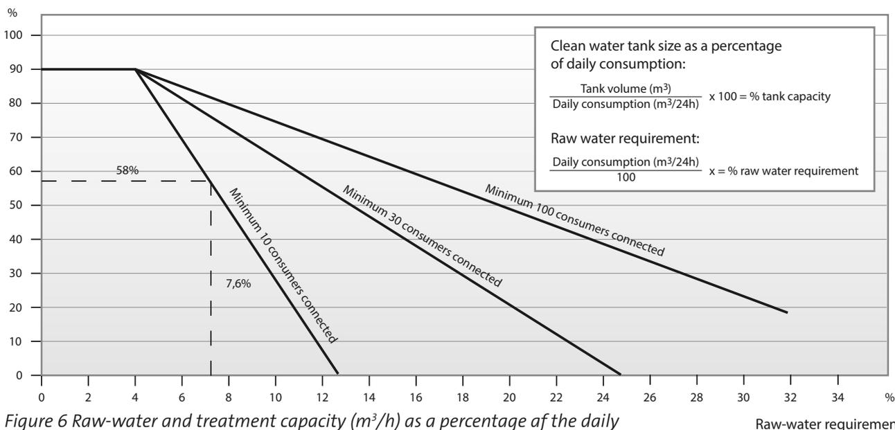
Figure 6 Raw-water and treatment capacity (m<sup>3</sup>/h) as a percentage of the daily consumption (m<sup>3</sup>/day)
