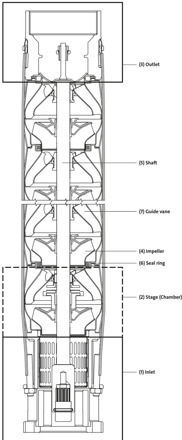
Figure 24 Submersible pump principle
