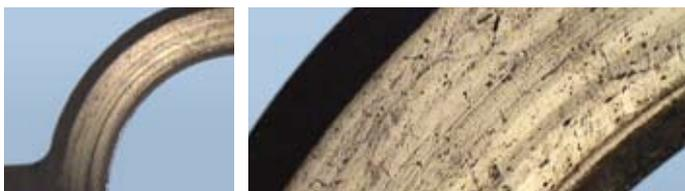
*Fig. 5.11: Normal wear on surface of tungsten carbide seal ring*
