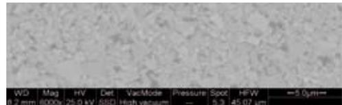
Fig. 3.6: Micrograph showing etched surface of tungsten carbide
