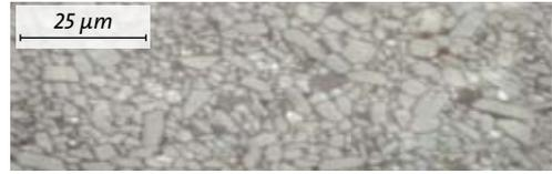
Fig. 3.4: Micrograph showing etched surface of alumina
