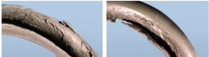
Fig. 5.19: O-rings extruded on account of high pressure
