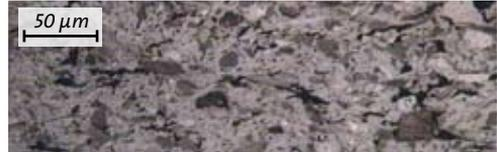
Fig. 3.2: Micrograph showing the material structure of resin-impregnated carbon graphite
