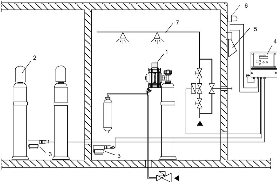
Fig. 2 Gas warning system, example of an application
