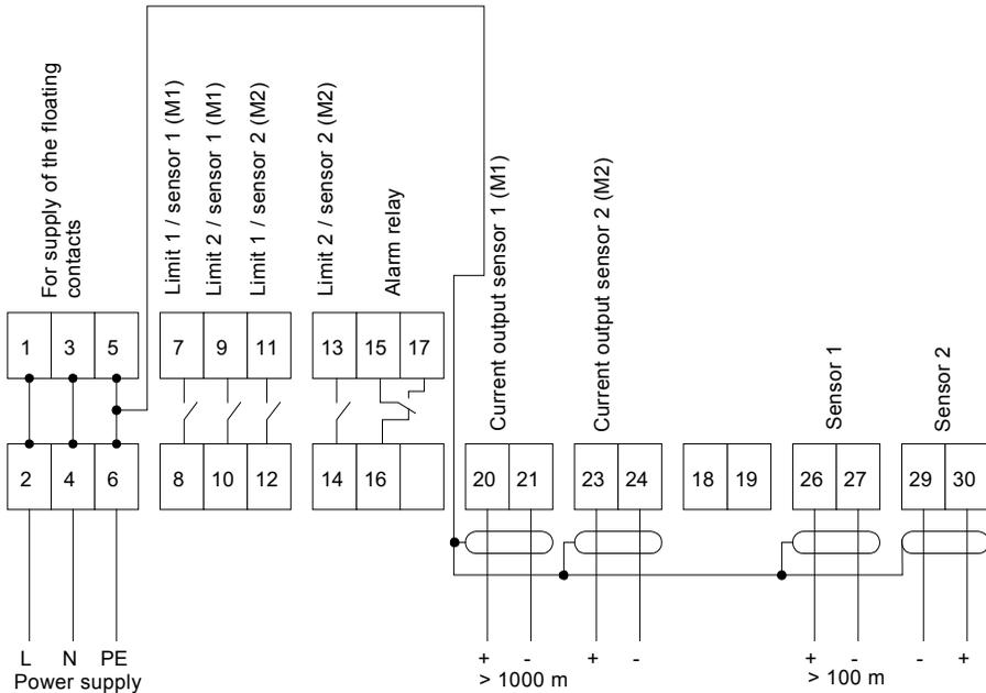
Fig. 6 Conex® DIS-G terminal
