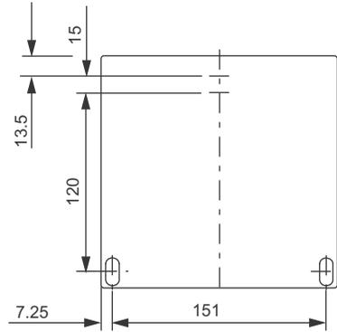
Fig. 4 Drilling diagram of the Conex® DIS-G
