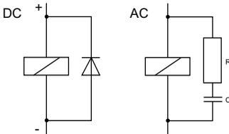
Fig. 7 Suppressor circuit DC / AC
