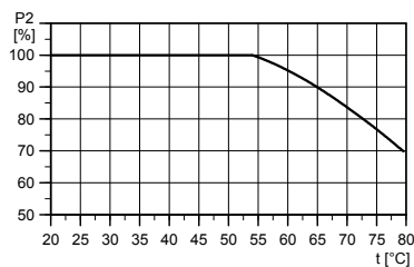
Fig. 13 Derating in relation to the ambient temperature
