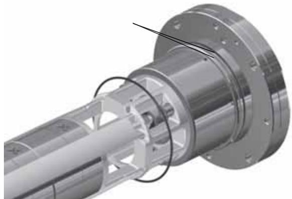
Fig. 29 Replacing the O-rings
