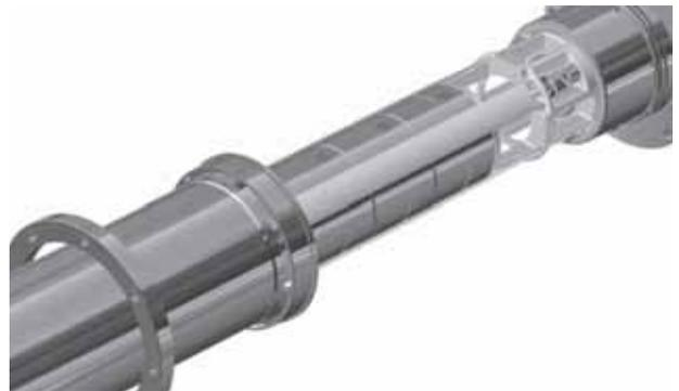
Fig. 28 Pulling out the pump
