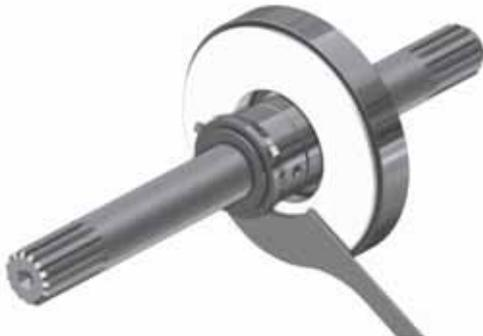
**Fig. 20** Tightening the shaft seal
