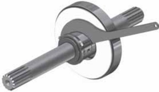
**Fig. 18** Loosening the shaft seal
