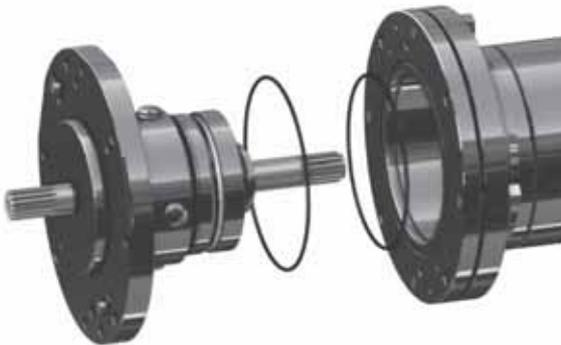
**Fig. 8** Removing O-rings
