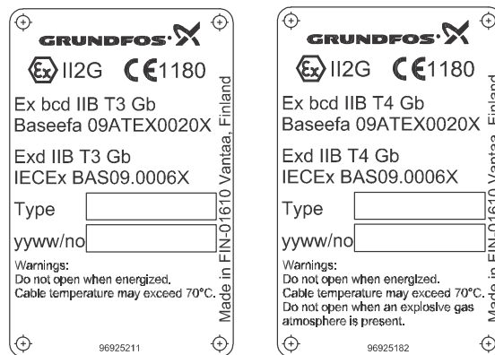
Fig. 3 Approval plates of explosion-proof pumps, T3 and T4 classification
