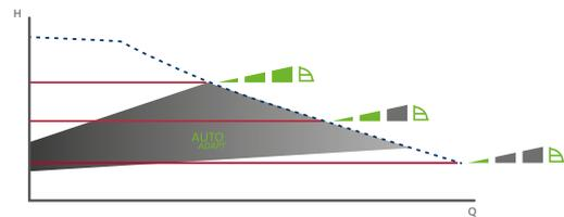
Fig. 23 Selection of pump setting for system type
