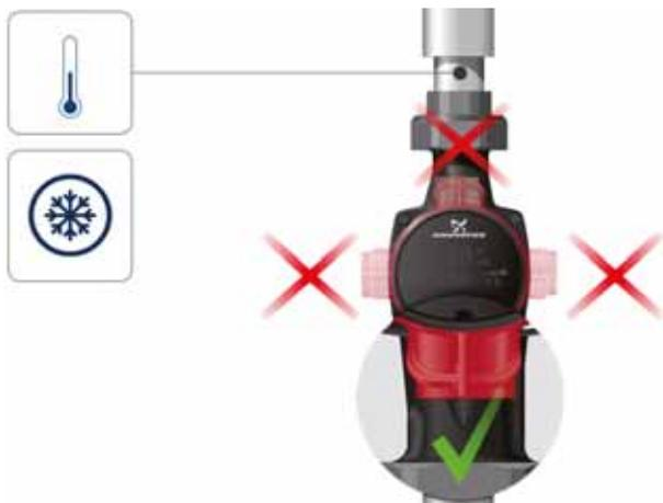
**Fig. 4** Control box position, air-conditioning and cold-water systems
