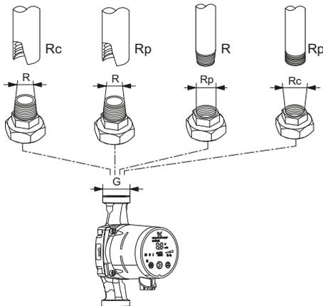
Fig. 43 G-threads and R-threads
