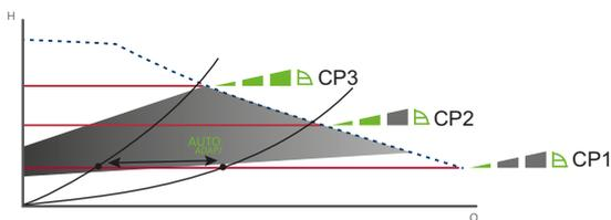
Fig. 26 Three constant-pressure curves or settings
