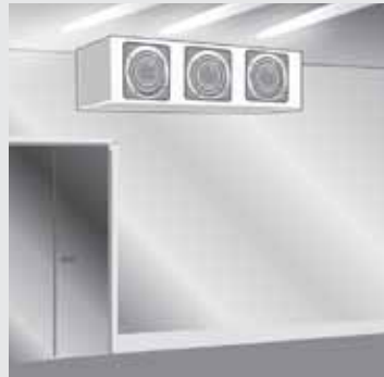
Fig. 6: Example of an evaporator in a cooling room.
