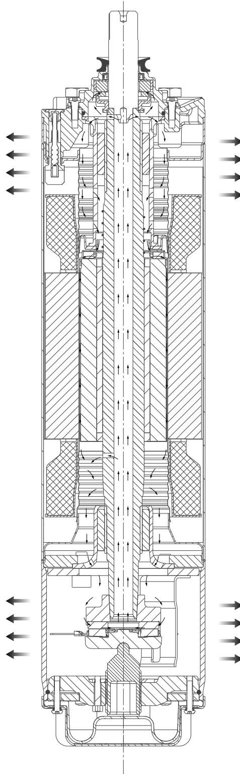
*Liquid circulation inside the motor*
