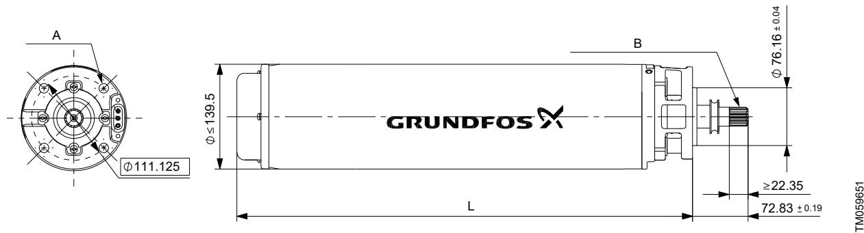
Dimensional drawing of the MS6000 and the MS6000P with flange extension
