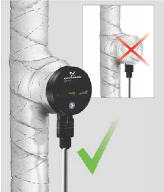
Fig. 4 Insulation of pump housing
