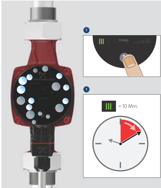
Fig. 5 Venting the pump
