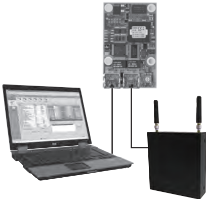
CIM 500 connected to PC and cellular router
