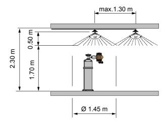
□ can fully sprinkle a circuit area of about 7.5 m² with fine water drops, if the height of the room is about 3.2 m.
