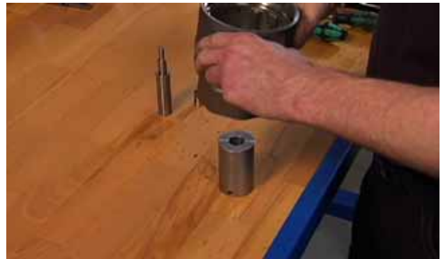
5. Position the valve casing upside down on the support tool from the punch set (pos. D).
