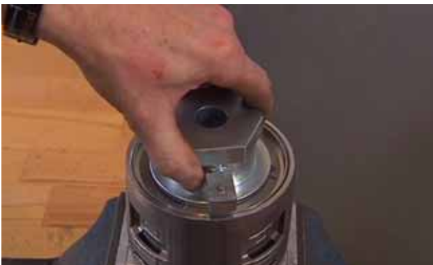
1. Fix the relieved valve casing (pos. 1a) upside down in a vice. 2. Fit the retainer ring tool (pos. S) in the retainer ring (pos. 203) for valve seat.
