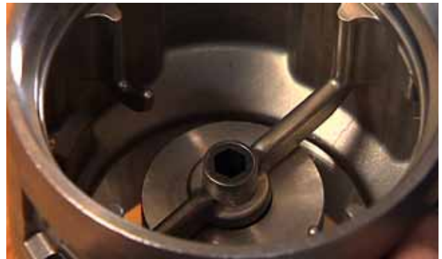
6. Centre the guide bearing (pos. 142a) with the hole in the support tool.
