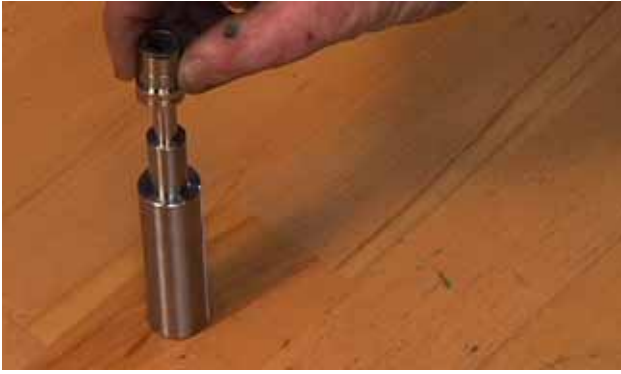
6. Fit the new guide bearing on the punch.
