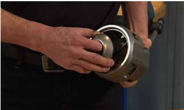
9. Insert the valve cup (pos. 2) into the valve casing.
