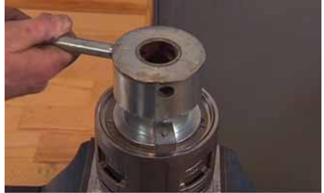
3. Place the spanner (pos. H) over the retainer ring tool and loosen the retainer ring. 4. Remove the retainer ring and valve cup (pos. 2).
