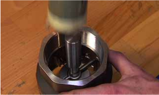
7. Position the new guide bearing in the valve casing. 8. Knock the guide bearing home with a plastic mallet.
