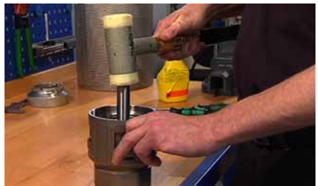
7. Position the punch tool in the centre of the guide bearing and knock it out with a plastic mallet.
