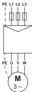
Fig. 9 Motors wound for direct-on-line starting
