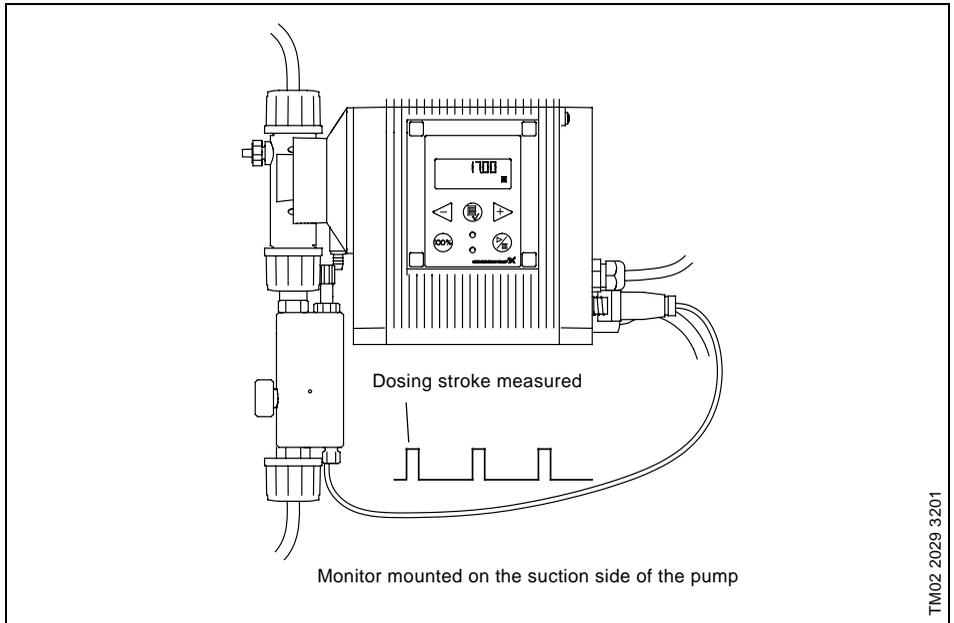
The dosing monitor is designed to monitor the dosing of liquids which may cause gas accumulation in the dosing head, thus stopping the dosing process even if the pump is still operating.
