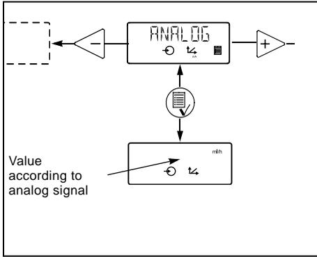
If 4-20 mA or 20-4 mA is selected and the signal falls below 2 mA, the pump will indicate a fault. This situation occurs if the connection is interrupted, for instance if the wire is damaged.
