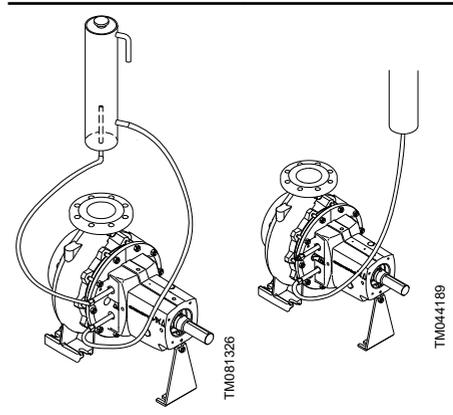
Pumps with double seal arrangements connected to an elevated vessel
