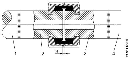
*Pipe connection using clamp couplings*
