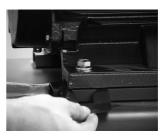
Tighten the screws to the correct torque. Go to step 3, and check the alignment once more.
