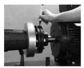
Hold a straightedge ruler against the coupling, and determine the inaccuracy, if any, with a feeler gauge.
