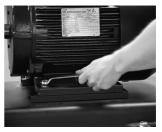
6. Insert shims with the required thickness.
