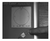
17. Turn the laser units to position 12 o'clock. Confirm on the control box.
