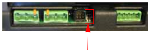
Indicator lights for operation and alarm on the control panel
