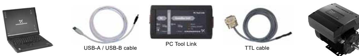
Fig. 15 Example of connection of a PC to the MGE-F
