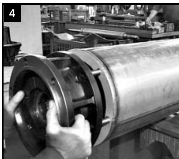
4 Mount lower bearing housing
