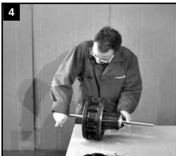
Use tool or an ordinary hydraulic press to insert bearing bushes
