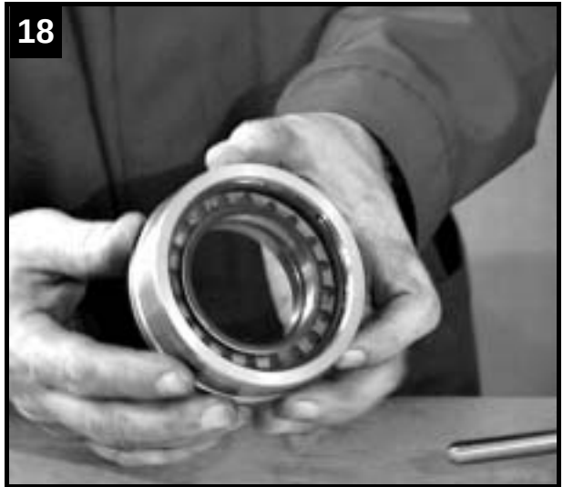
Correctly fitted seal ring
