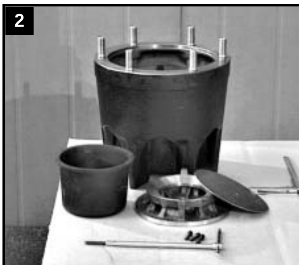
Thrust bearing housing parts and tools
