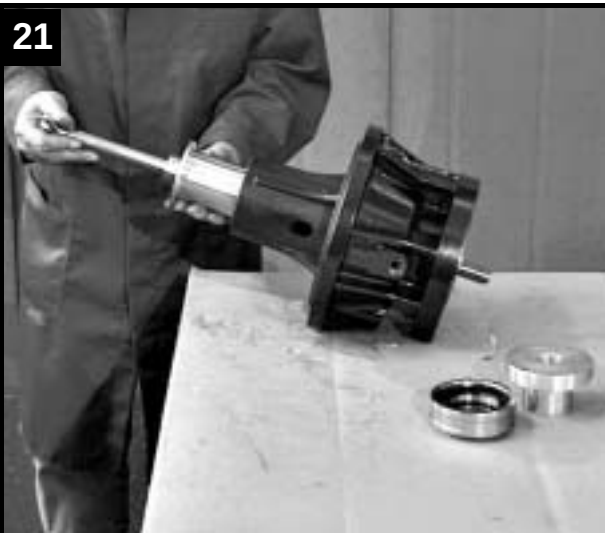
Fit tool in upper motor bearing housing
