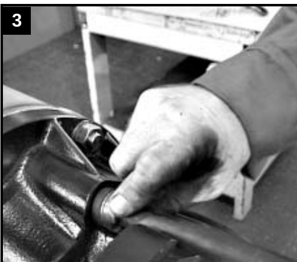
Press cable glands into bearing housing
