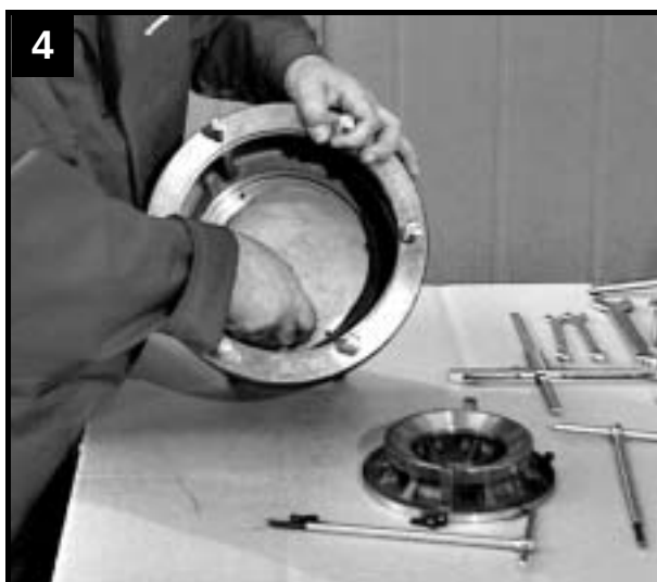
Fit diaphragm plate
