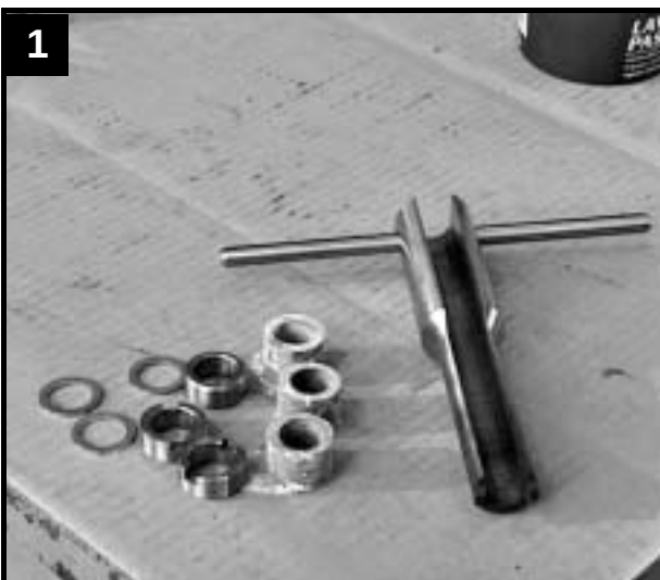
Cable gland rings, cable grommets, cable glands and special tool
