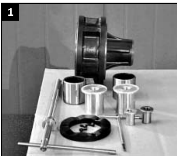
Lower motor bearing housing parts and tools
