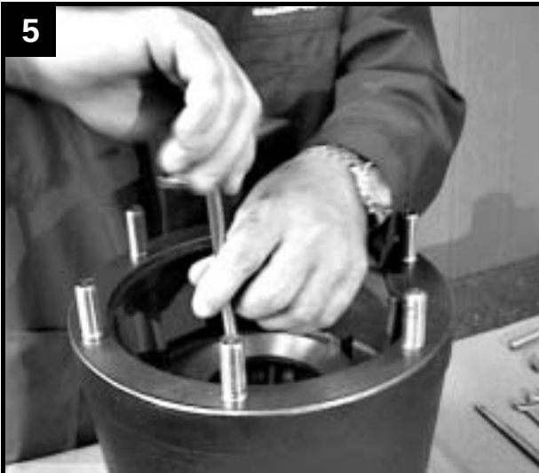
Fit stationary disc for thrust bearing
