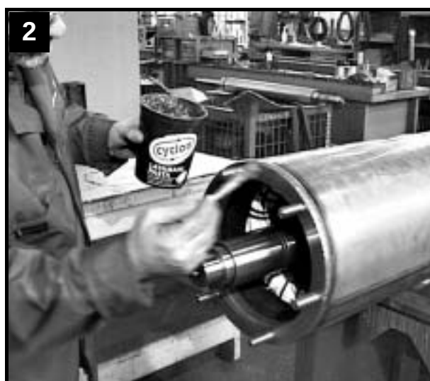
2 Grease seal surface on stator housing
