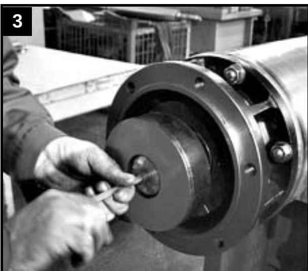
Fit washer and screw
