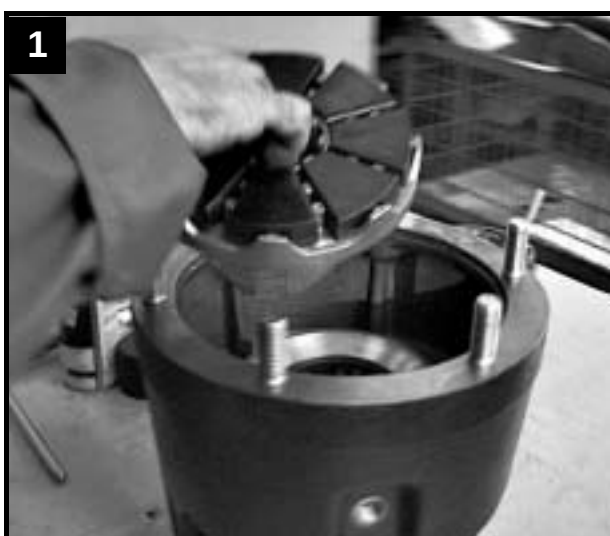
Fit thrust bearing pad assembly in thrust bearing housing
