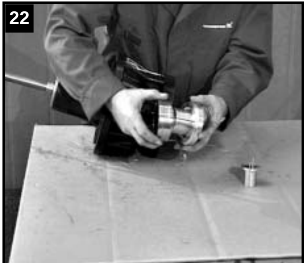
Place housing for seal ring on tool
