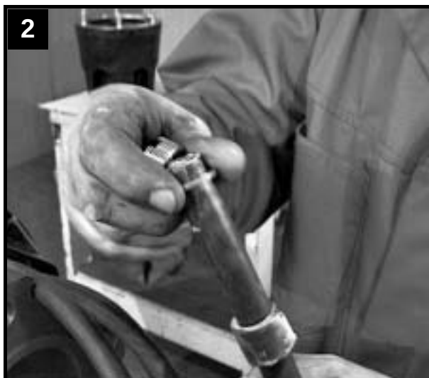
Fit cable grommet, cable gland ring and cable gland on cables
