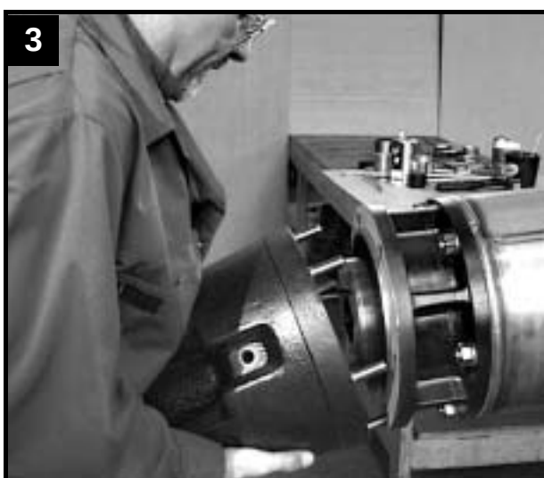
Mount thrust bearing housing
