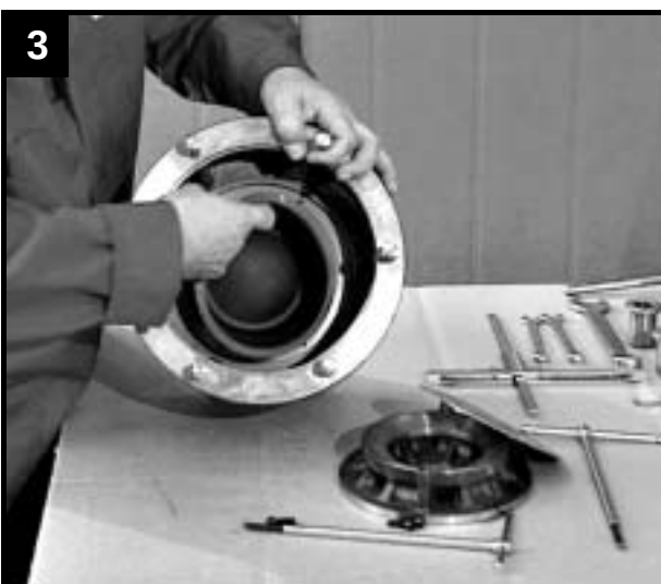
Insert diaphragm in thrust bearing housing
