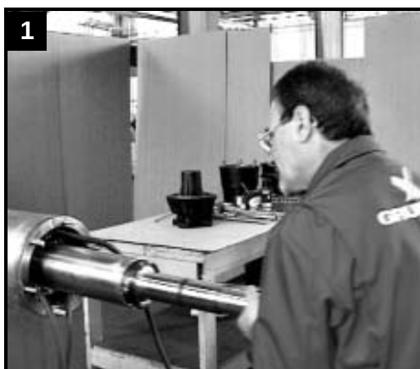
1 Fit rotor. Be careful not to damage windings
