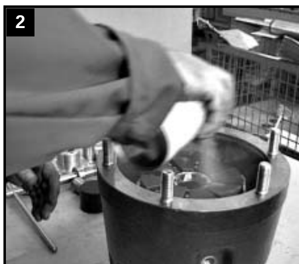
Lubricate thrust bearing pads with silicon oil
