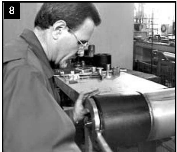
Tighten bottom bearing housing with special tool
