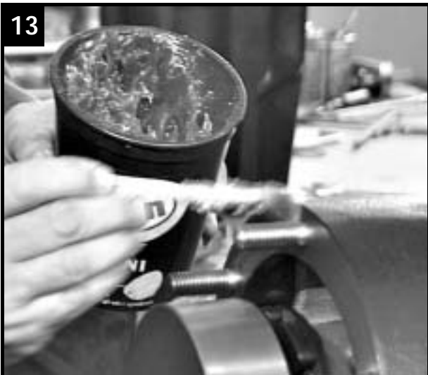
13 Grease surface for gasket
