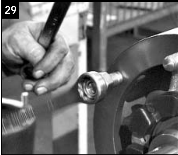
Long thread ends must point outwards
