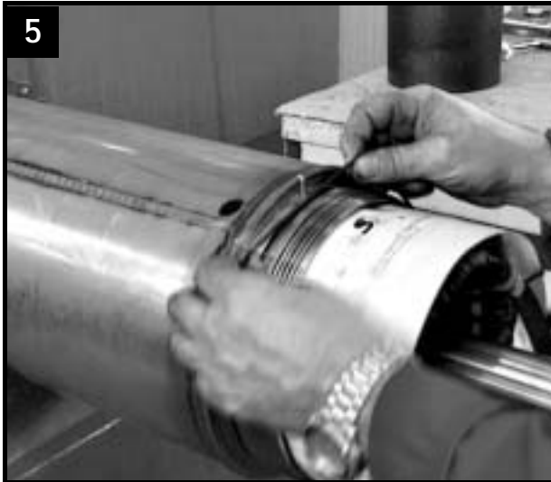
Fit O-ring at upper end of stator
