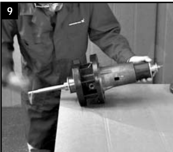
Fit bearing bushes by means of tool or an ordinary hydraulic press
