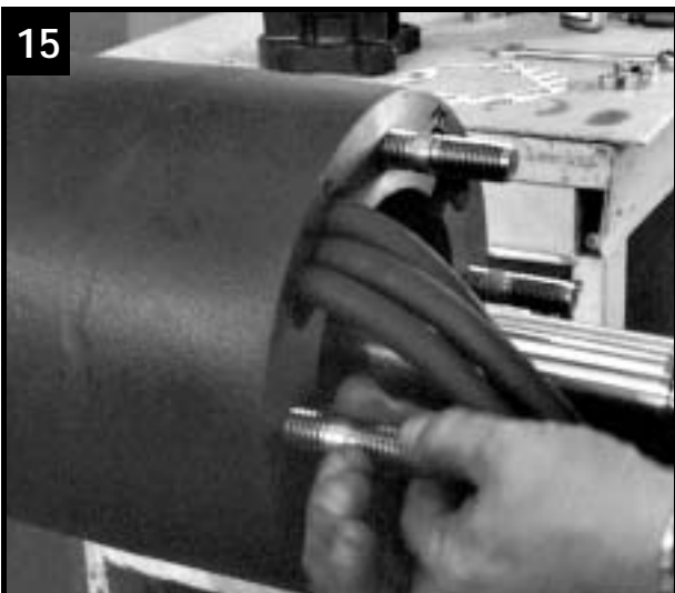
15 Fit studs in upper motor casing
