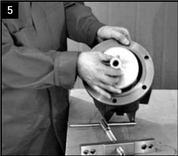
Fit thrust part of special tool
