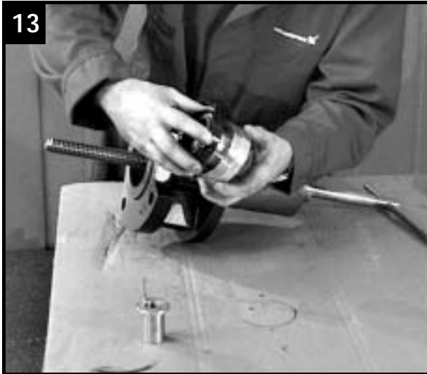
13 Fit radial shaft seal rings on housing and special tool
