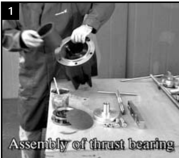
Fit breather diaphragm in thrust bearing housing
