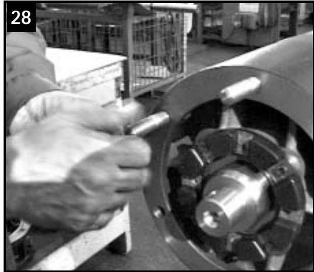
28 Fit studs in lower bearing housing
