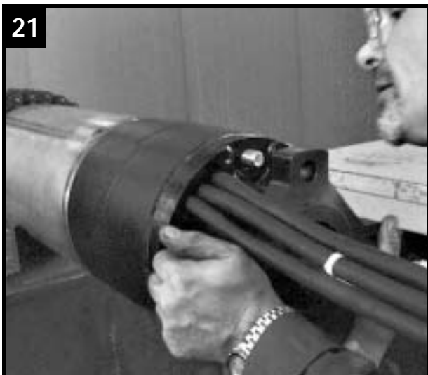
21 Mount upper bearing housing
