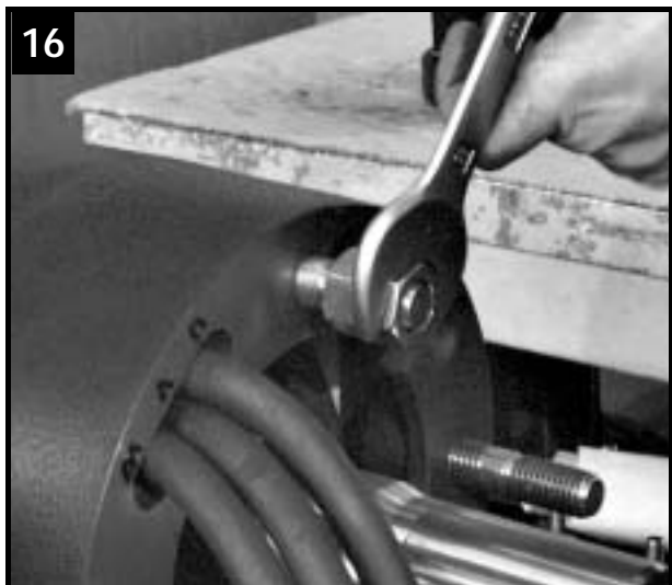
16 Long thread end pointing outwards
