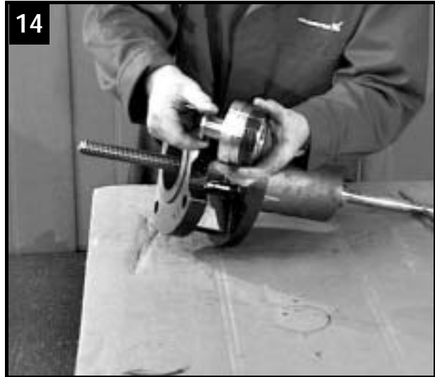
14 Fit threaded part of special tool
