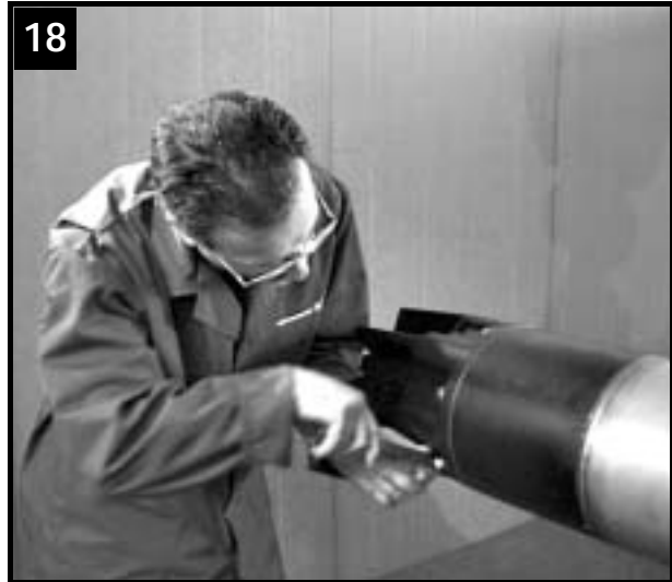
18 Mount thrust bearing housing on bearing housing. Fit spacers and nuts
