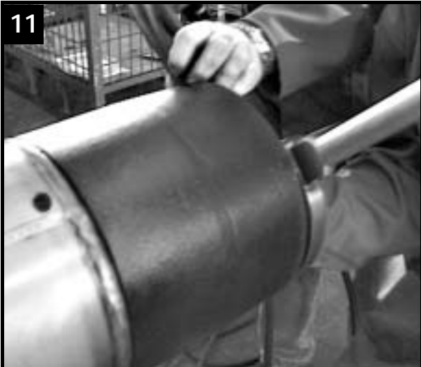
11 Mount upper motor casing and tighten. Note: left-hand thread
