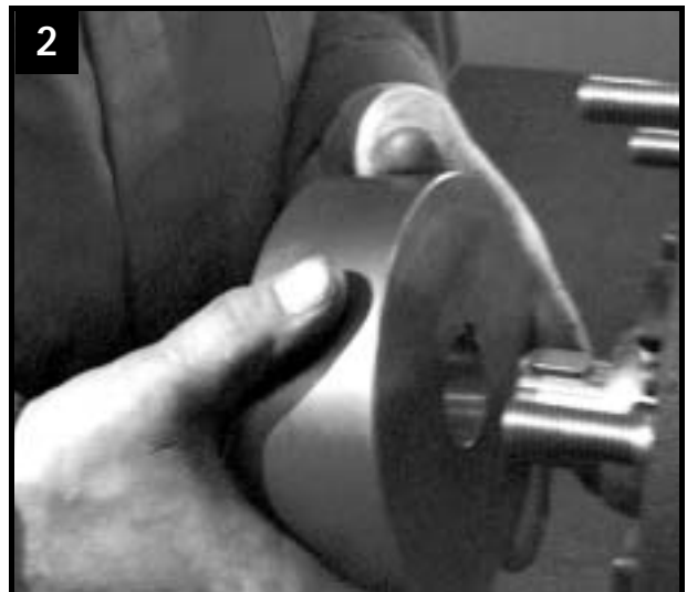
Fit thrust bearing plate
