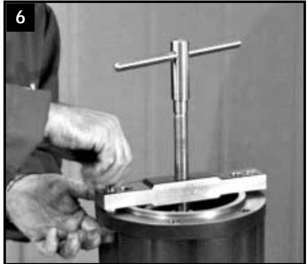
Fit spindle part of tool on thrust bearing housing
