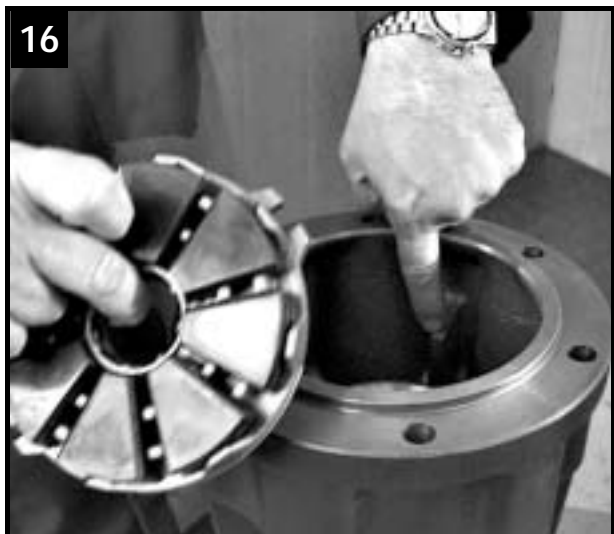
16 Must be engaged with rib inside thrust bearing housing
