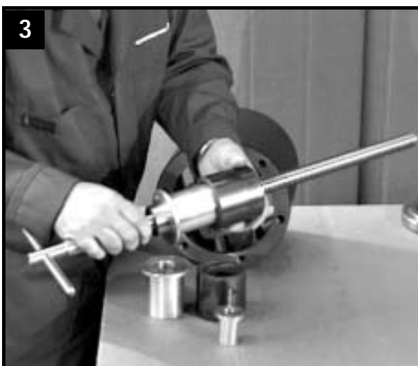
Fit first bearing bush on tool
