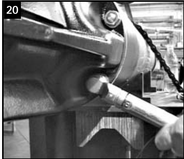
20 Tighten nuts at prescribed torque
