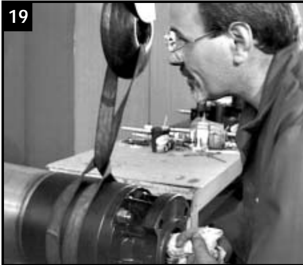
19 Check free rotation of rotor
