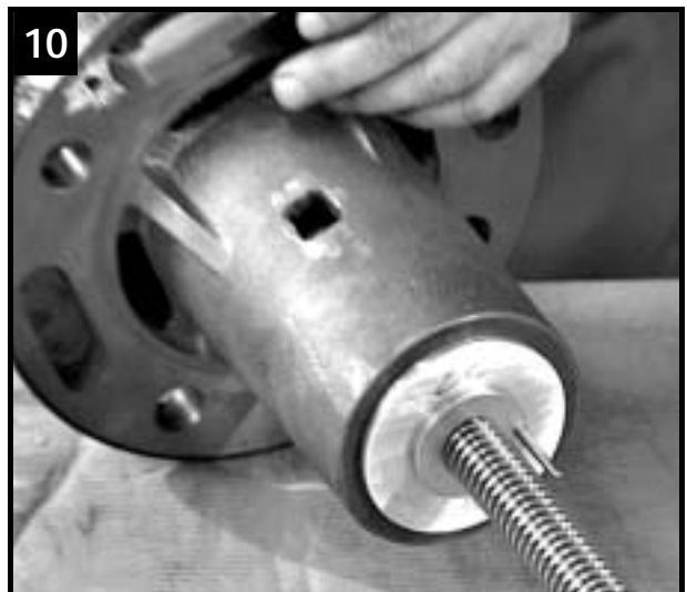
Bearing bushes are pressed into bottom position
