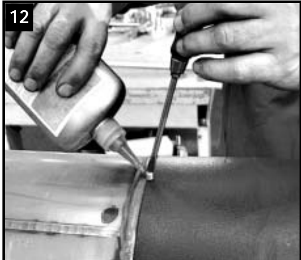
12 Lock upper motor casing with screw and Loctite
