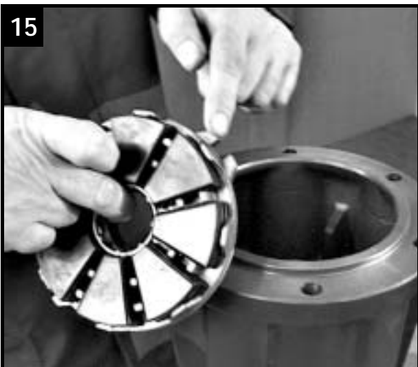
15 Note position of notch of pad assembly
