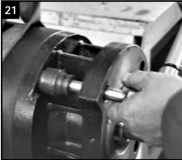
21 Tighten nuts in upper motor bearing housing at prescribed torque
