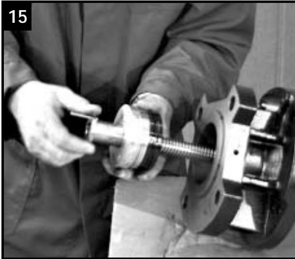
15 Screw parts on spindle
