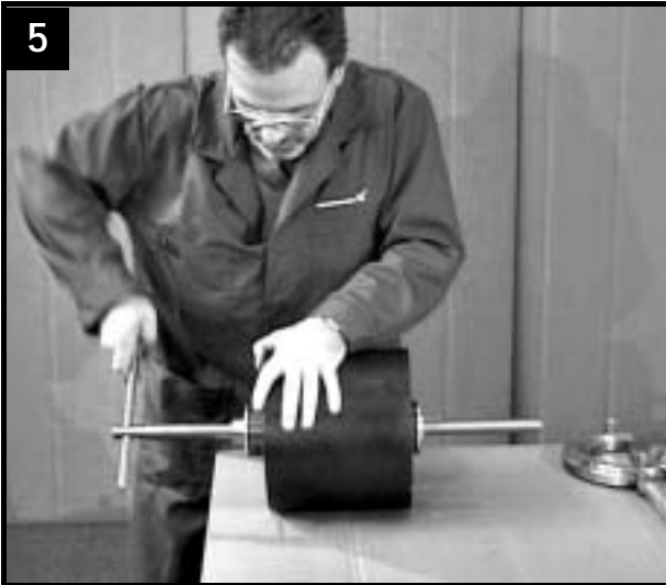
Use special tool or an ordinary hydraulic press to fit bearing bushes
