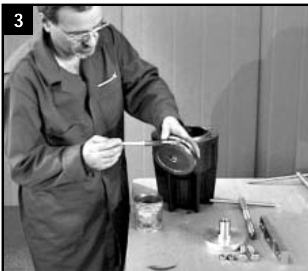
Grease stationary disc for thrust bearing to ease assembly
