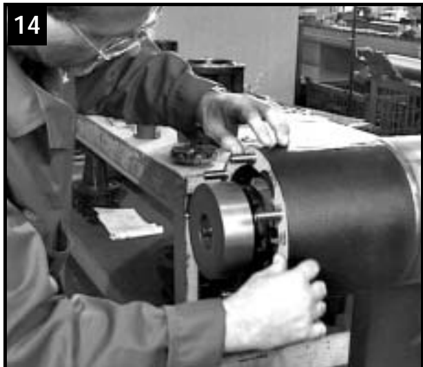
14 Fit gasket on bearing housing
