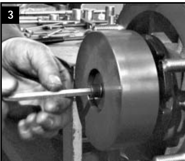
Fit spacer and tighten screw
