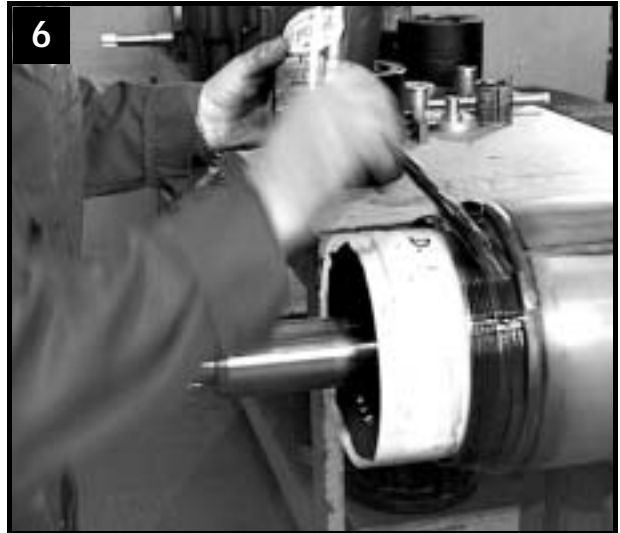
Grease thread and O-rings to ease assembly
