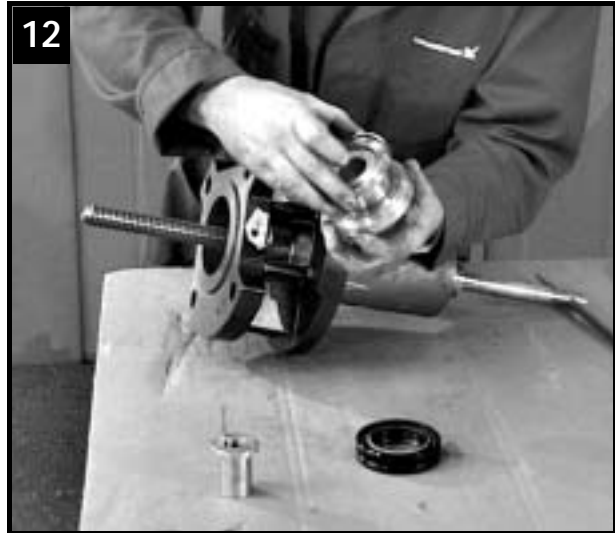
12 Fit housing for radial shaft seal rings on special tool
