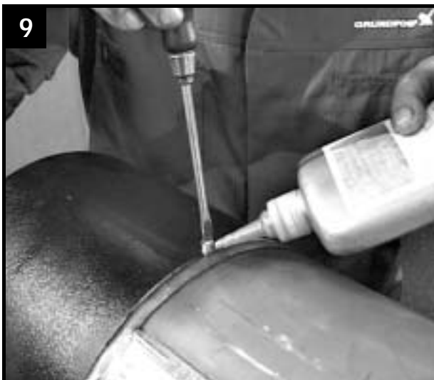
Lock bottom bearing housing with screw and Loctite
