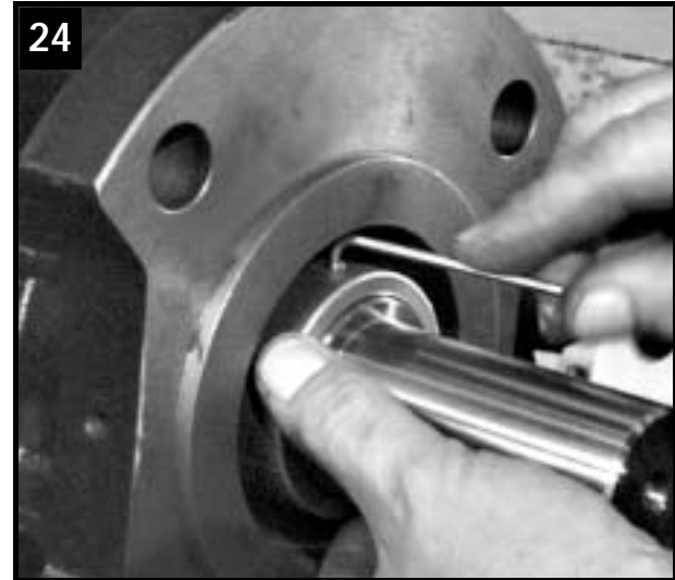
Tighten Allen screw in sand guard
