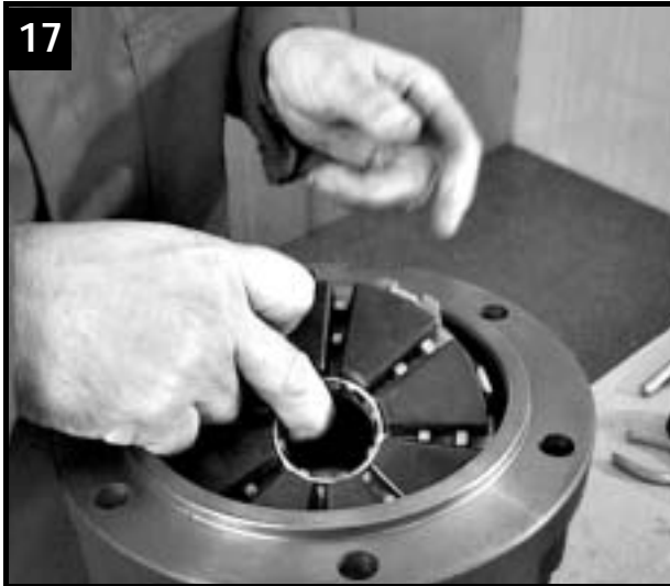
17 Fit thrust bearing pads in correct position
