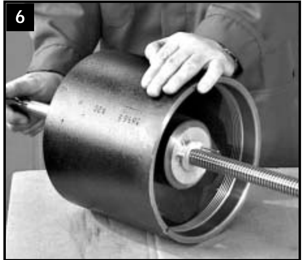
Press bearings into bottom position
