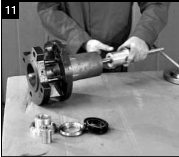
11 Prepare fitting of radial shaft seal rings
