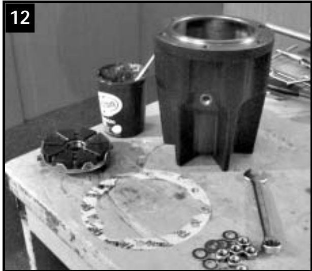
12 Thrust bearing pad, housing and gasket
