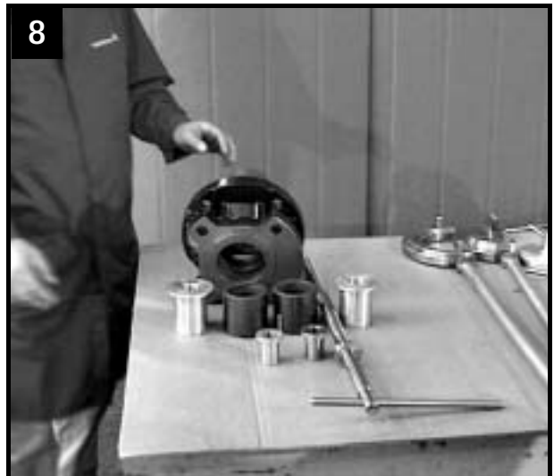
Upper bearing housing with bearing bushes and special tools
