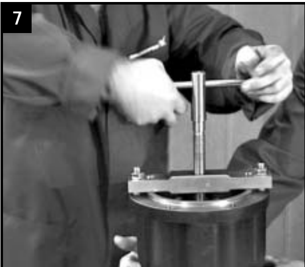
Press stationary disc of thrust bearing into bottom position
