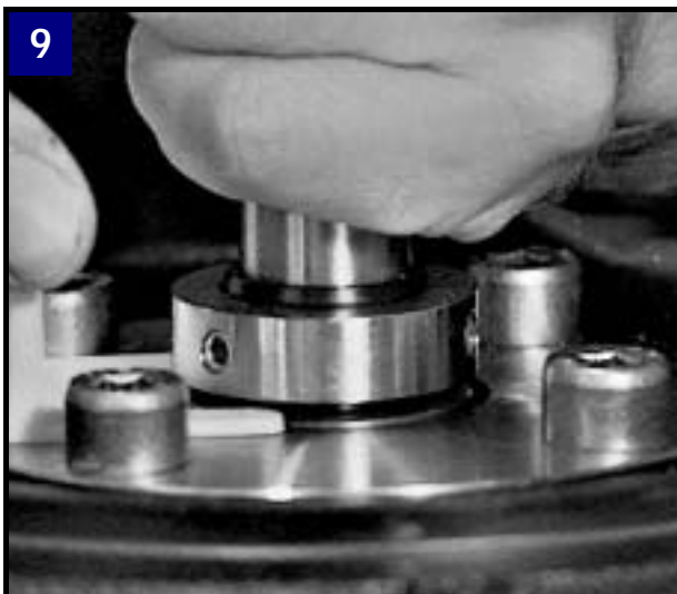
9 Raise shaft and insert forked distance piece under seal driver.
