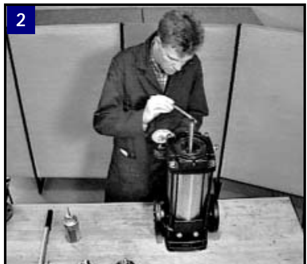
2 Grease shaft end with Unisilicone L641 to prevent damage of O-ring.
