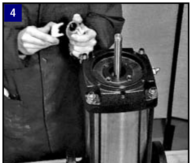
4 Remove forked distance piece from shaft seal.
