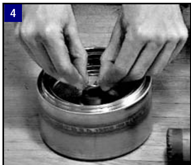
Place new bush/bearing in bearing retainer and fit lock ring.
