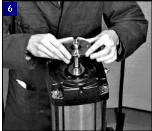
6 Fit seal carrier.
