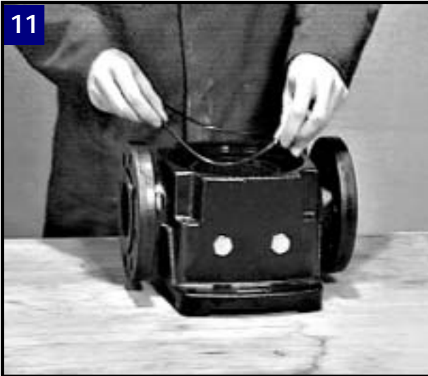
11 Check that groove for O-ring is clean. Fit O-ring properly in groove.
