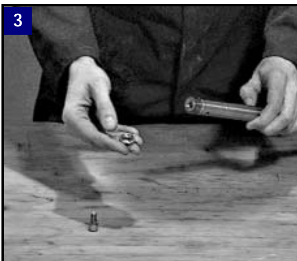
3 Fit washer. Important that teeth on washers interlock.
