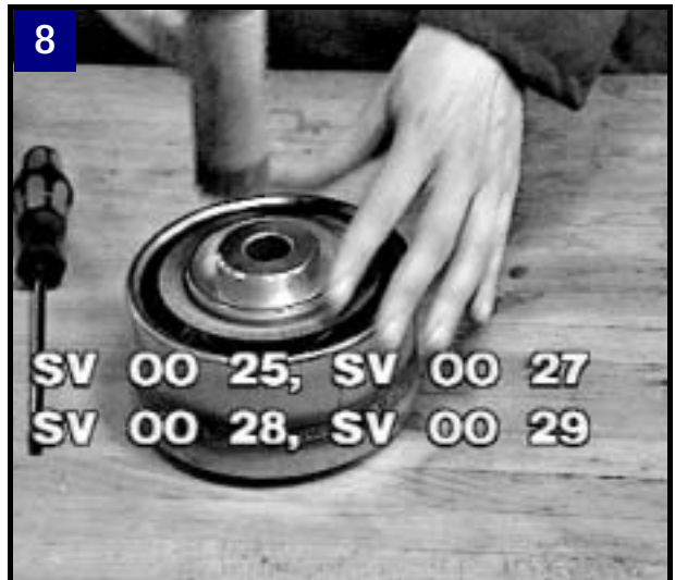
Knock retainer in position using one of the tools mentioned. See Service Manual.
