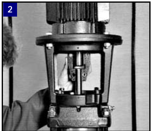
2 Fit coupling so that pump shaft end is level with bore in coupling.
