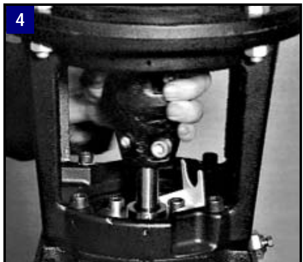
4 Remove forked distance piece (place under bolt head) and ensure trouble-free rotation.
