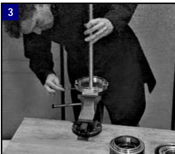
Place proper assembly tool in vice. Secure shaft by means of pin.
