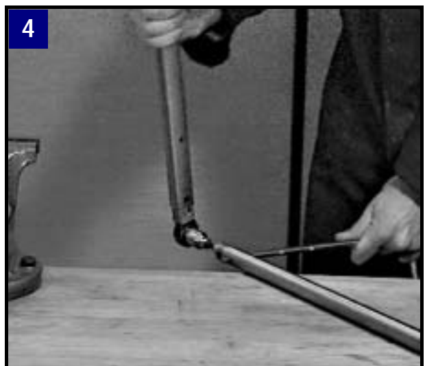
4 Fit Allen screw with lock washer and tighten at prescribed torque.
