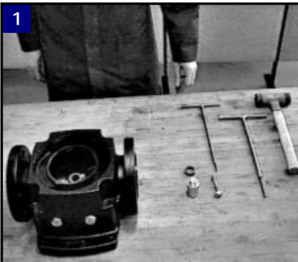
Parts and tools for replacement of bearing in base.
