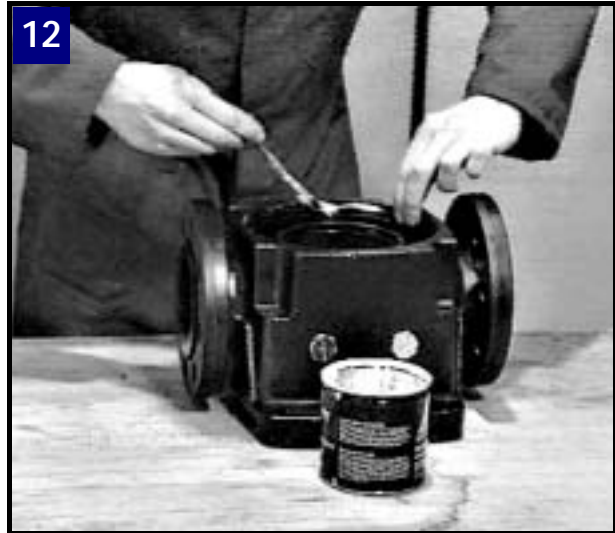
12 Grease O-ring with Unisilicone L641 to ease fitting of sleeve.
