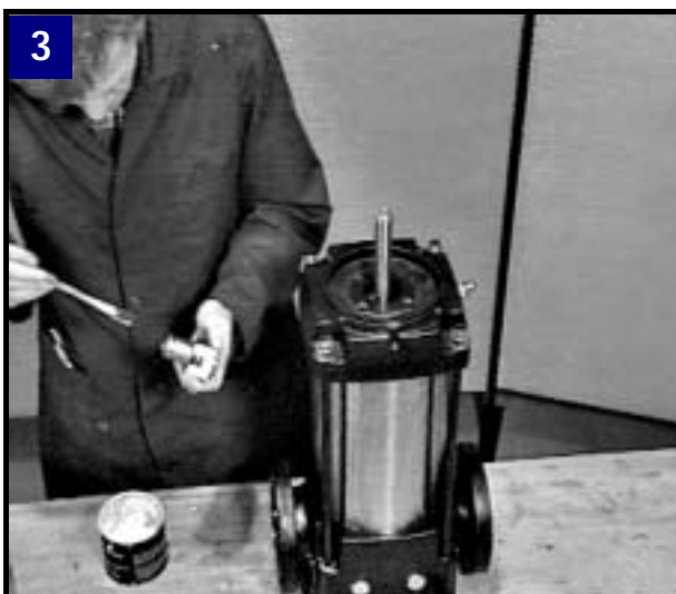
3 Grease O-rings on shaft seal with Unisilicone L641.
