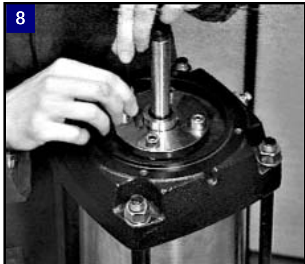
8 Ensure free movement of shaft. Tighten seal driver and check free rotation again.
