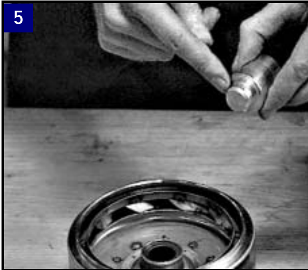
Use tool SV0015 to fit bush/bearing.
