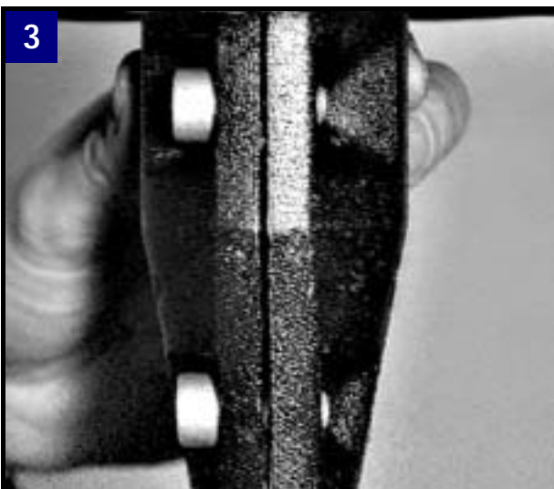
3 Tighten one side at a time so that air gap between the two halves is the same.
