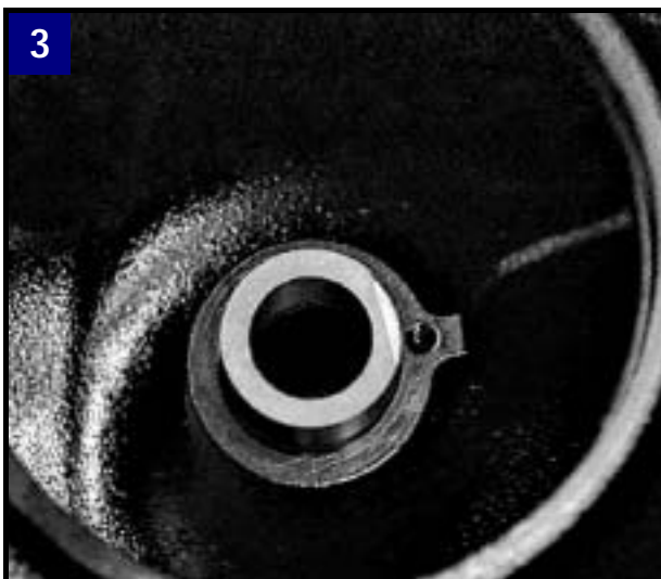
Bottom bearing recess must point upwards and towards M6 threaded hole in base.
