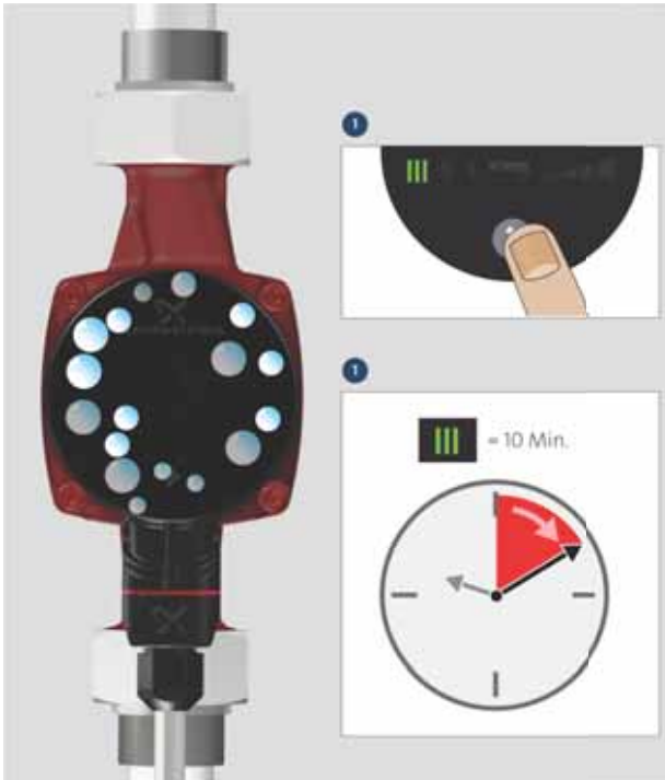
Fig. 5 Venting the pump
